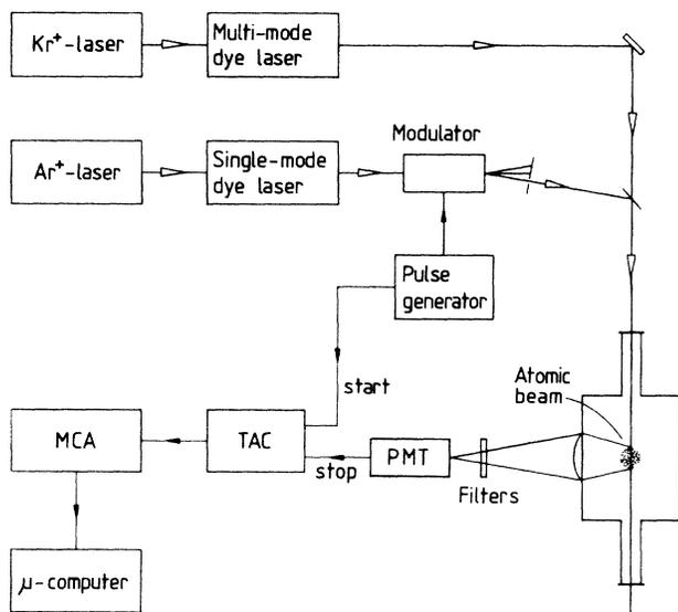
FIG. 2. Experimental setup for the PUMOLS measurements.
