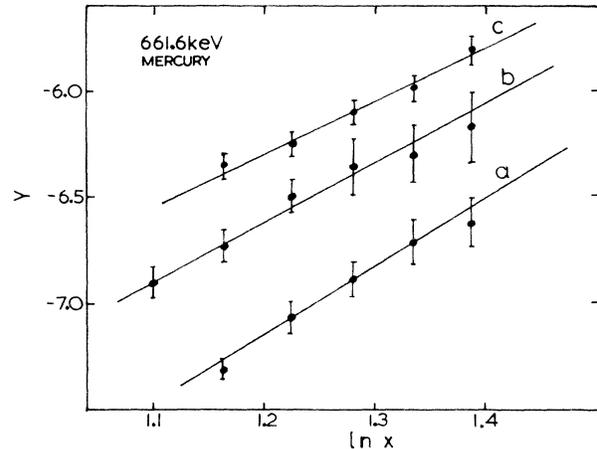
FIG. 6. Least-squares fits through the values of the quantity  $Y = \ln[(I/I_0 e^{-\mu x}) - 1] - \mu x$  plotted as a function of  $\ln x$ . (a)  $\mu t = 5.5$ , (b)  $\mu t = 4.4$ , (c)  $\mu t = 3.3$ .  $Y$  is obtained from the curves in Fig. 4.
