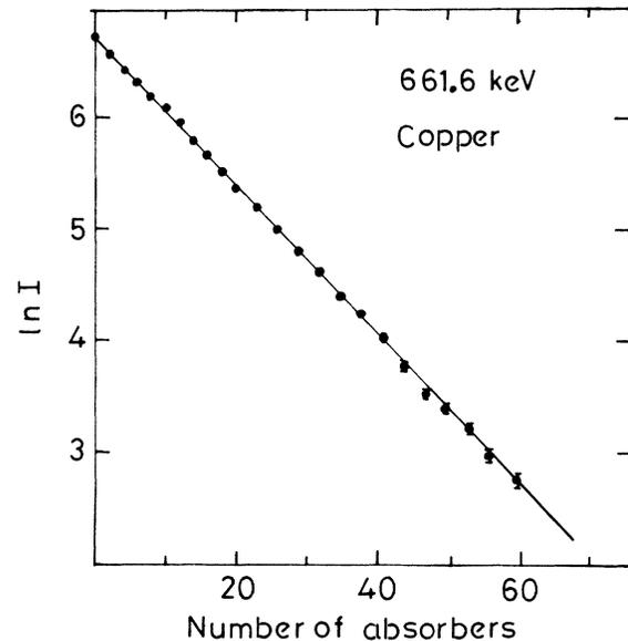
FIG. 3. Attenuation curve for the copper absorber. The copper absorber thickness is  $0.926 \text{ g/cm}^2$  per sheet. The error bars shown are the statistical errors. For the initial few points, the errors are less than or equal to the size of the points.
