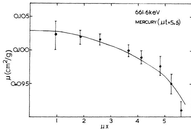
FIG. 5. Variation of  $\mu$  of mercury with  $\mu x$  for  $\mu t = 5.5$ .
