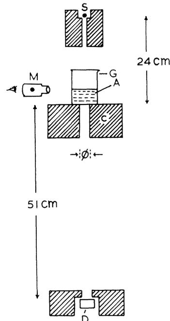
FIG. 1. Experimental arrangement for  $^{137}\text{Cs}$   $\gamma$ -ray attenuation measurements with copper and mercury absorbers.
