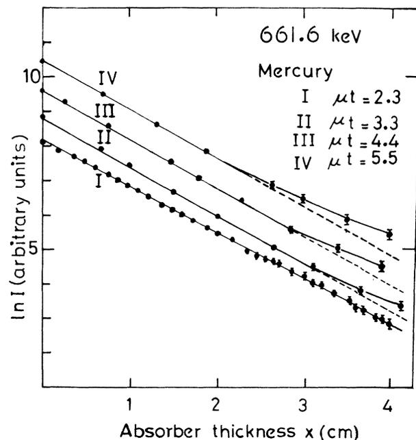
FIG. 4. Attenuation curves for the mercury absorber, for various values of  $\mu t$ . The solid line for  $\mu t = 2.3$  (curve I) is the least-squares fit through the experimental points. For other  $\mu t$  values, the solid lines are just visual fits. The dashed extensions of these solid lines show the expected linear variation. Wherever the statistical errors are greater than the size of the points, they are indicated by the error bars.
