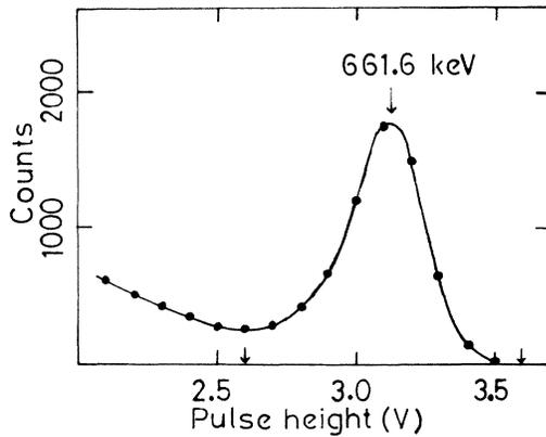
FIG. 2. Pulse-height spectrum of  $^{137}\text{Cs}$   $\gamma$  rays obtained with a  $2 \times 1\frac{1}{2}$ -in.<sup>2</sup> NaI(Tl) detector and a SCA. The arrows on the x axis show the window setting used.
