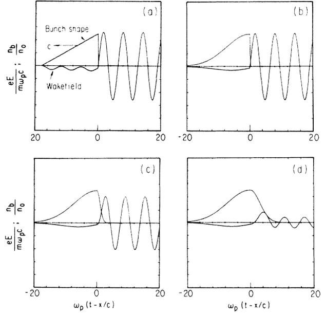
FIG. 2. Numerical solutions of 1D wake fields produced by various bunch shapes: (a) Triangular bunch; (b) Gaussian rise,  $\sigma_r = 7.2c/\omega_p$ . Gaussian fall,  $\sigma_f = 0.1c/\omega_p$ ; (c)  $\sigma_r = 7.2c/\omega_p$ ,  $\sigma_f = 1c/\omega_p$ ; (d)  $\sigma_f = 3c/\omega_p$ .
