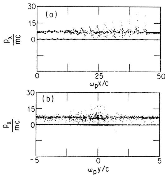
FIG. 4. Phase space of accelerated particles in 2D simulations of Fig. 3 at  $t=90\omega_p^{-1}$ . (a)  $p_x$  vs  $x$ , (b)  $p_y$  vs  $y$ . Particles were initially uniformly distributed in space behind the driving bunch with energy  $\gamma=7=\gamma_b$  and density  $0.005n_b$ .
