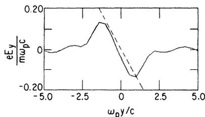
FIG. 6. Focusing field ( $E_y$  vs  $y$ ) from the 2D computer simulations ( $t = 45 \omega_p^{-1}$ ,  $x = 41.7c / \omega_p$ ) and the corresponding linear prediction from Eq. (11).
