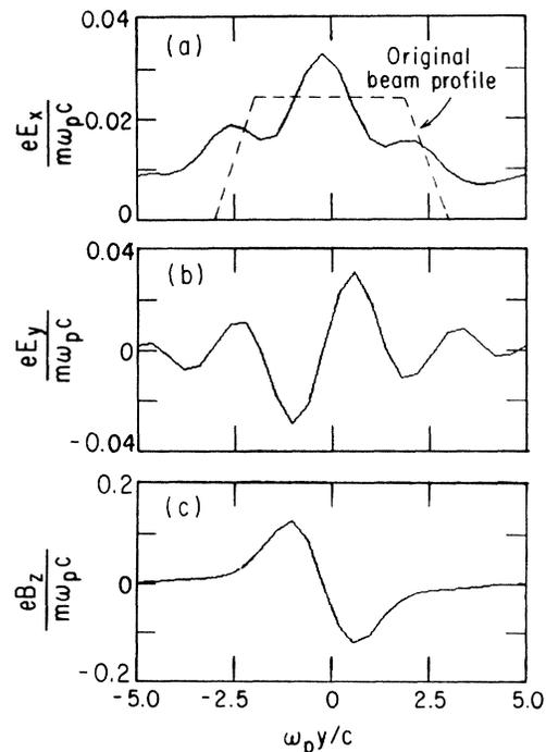
FIG. 8. Fields in the driving bunch ( $t = 45 \omega_p^{-1}$ ,  $x = 41.7c / \omega_p$ ). (a)  $E_x$  vs  $y$ , (b)  $E_y$  vs  $y$ , (c)  $B_z$  vs  $y$ .
