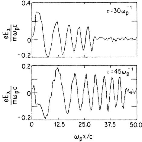
FIG. 10. One-dimensional simulations of wake fields produced in a linear plasma-density gradient at (a)  $t=30\omega_p^{-1}$  and (b)  $t=45\omega_p^{-1}$ . The plasma density at the right boundary is four times that at the left boundary ( $n_0$ ); the driving bunch was a doorstep rising to  $0.2n_0$  in  $1\lambda_p$ .
