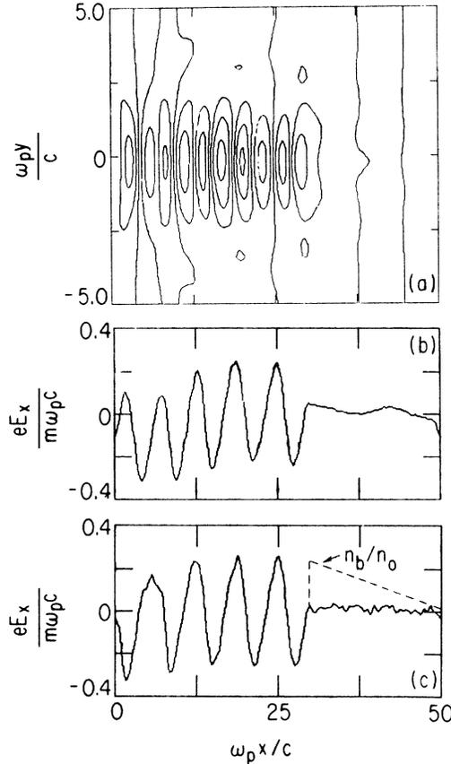
FIG. 3. Plasma wakes in simulations. (a) Contours of equipotential in 2D simulation; (b) electric-field slice down the  $y=0$  axis of (a); (c) electric field from a 1D simulation corresponding to (b). For all cases  $t=30\omega_p^{-1}$ , bunch density was  $\rho_b(\xi)=0.01n_0$  for the first  $\lambda_p/4$  and rose to  $0.2n_0$  over the next  $3\lambda_p$  [as indicated in Fig. 3(a)]. For the 2D cases, the bunch width was trapezoidal over  $y=-2c/\omega_p$  to  $+2c/\omega_p$ .
