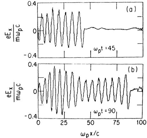
FIG. 7. Slice plots of 2D wake fields ( $E_x$  vs  $x$  at  $y=0$ ) at (a)  $t = 45 \omega_p^{-1}$  and (b)  $t = 90 \omega_p^{-1}$  showing changes in the wake-field amplitude.
