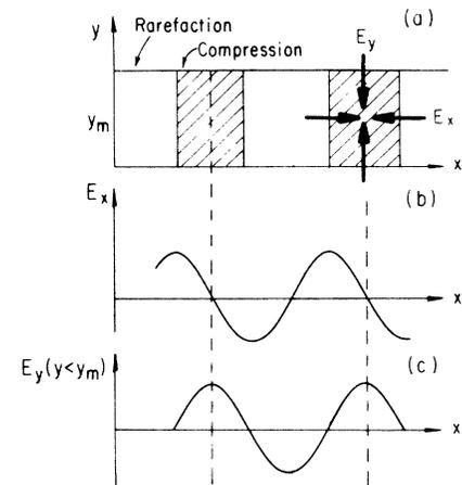
FIG. 5. In finite-width plasma waves, electric fields point toward the density compressions as shown in (a) giving rise to the longitudinal and radial fields shown in (b) and (c), respectively.
