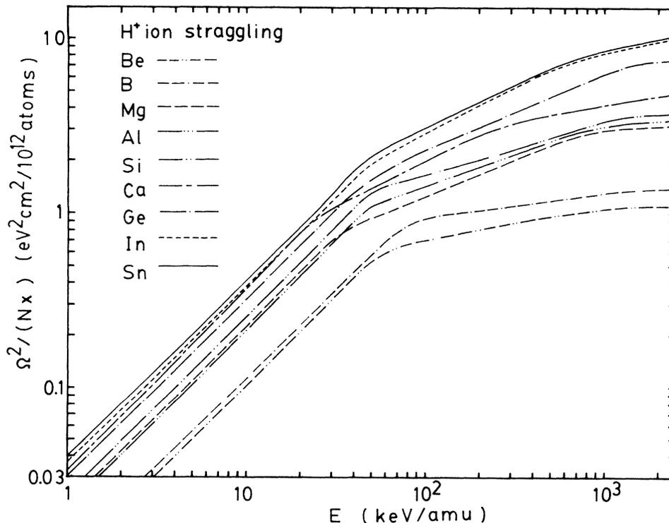
FIG. 1. The collisional straggling of a  $H^+$  ion incident on solids calculated from Eq. (2.9) with the solid LEDM.
