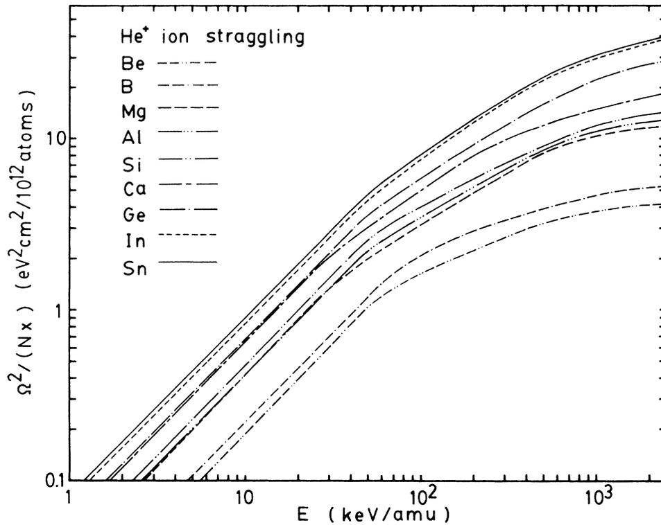
FIG. 2. The collisional straggling of a  $\text{He}^+$  ion incident on solids calculated from Eq. (2.9) with the solid LEDM.
