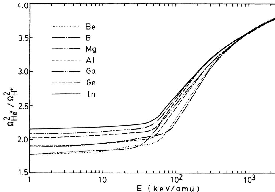
FIG. 3. The ratio of the collisional stragglings,  $\Omega_{\text{He}^+}^2 / \Omega_{\text{H}^+}^2$ , calculated for solids.
