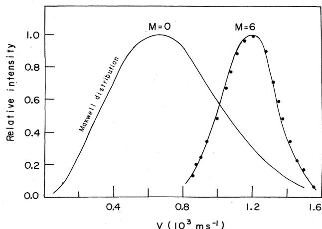
FIG. 3. Closed circles are the measured speed distribution of one Na jet. Note excellent fit to distribution calculated from a Mach 6 supersonic jet at  $500^\circ\text{C}$ .
