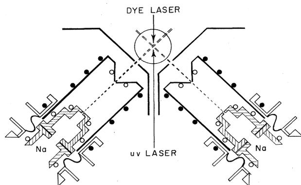
FIG. 2. Schematic diagram of the apparatus. Open circles indicate heating elements; closed circles are cooling elements.
