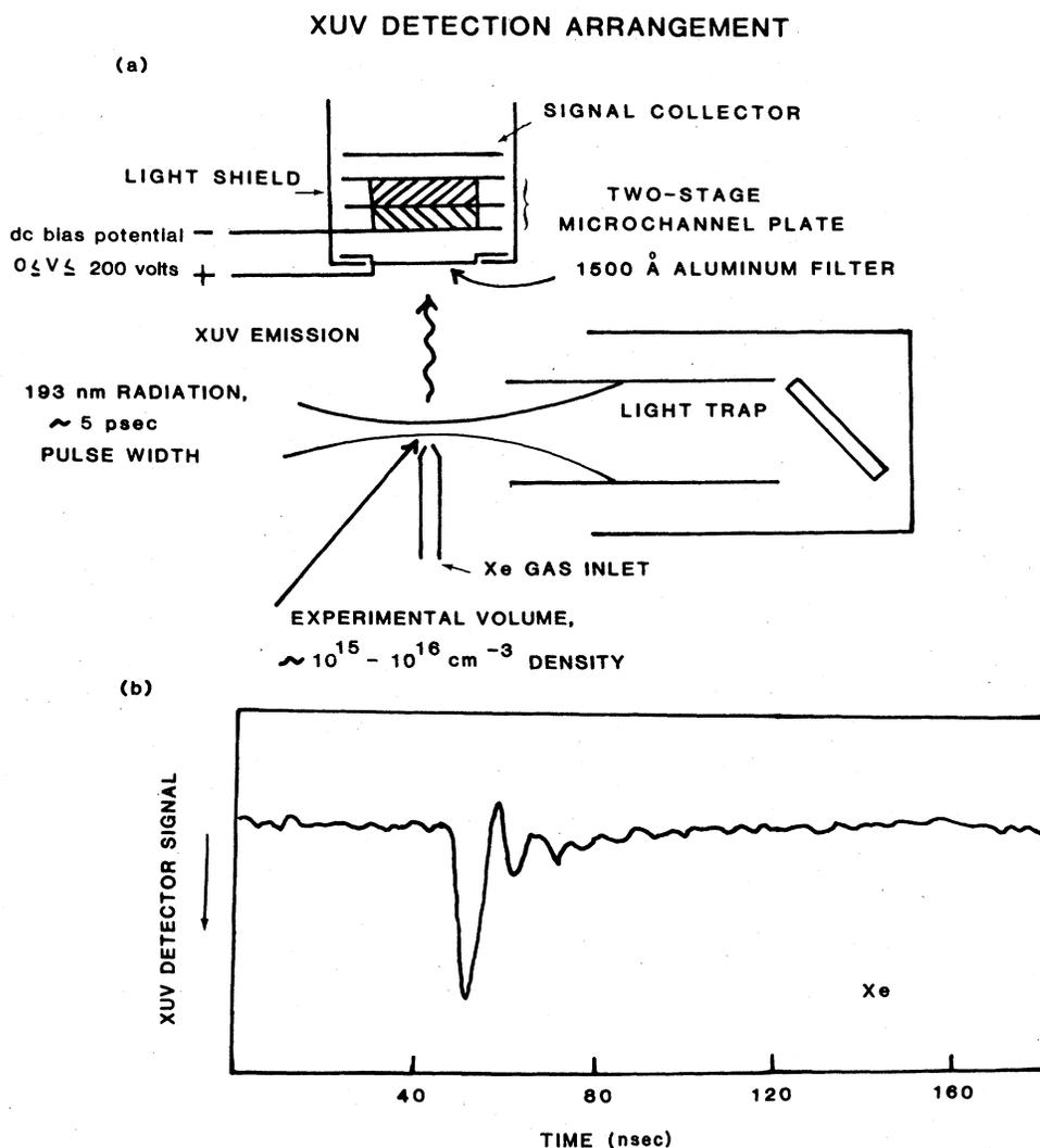
FIG. 10. (a) Experimental arrangement used to detect xuv radiation from highly excited atoms excited by 193-nm radiation at an intensity of  $\sim 10^{16}$ – $10^{17}$  W/cm<sup>2</sup>. (b) xuv signal observed from xenon in the 10–100 eV range with  $\sim 100$ -V bias between the aluminum filter and the microchannel plate; some ringing of the detector circuit is evident.
