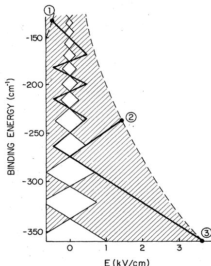
FIG. 5. Methods by which Na atoms ionize in an 8-GHz field. ① the  $1/3n^5$  ionization of  $|m|=0$  and 1 states, ② the  $1/21n^4$  ionization of the  $|m|=2$  states, ③ the  $1/9n^4$  ionization of the  $|m|=2$  states.
