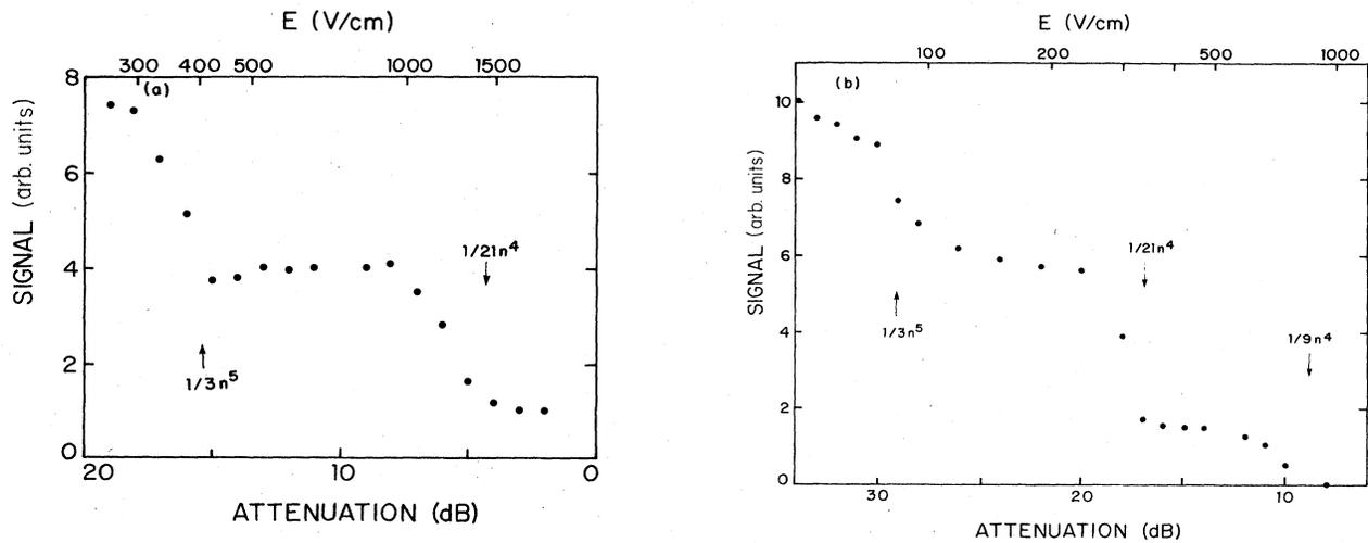
FIG. 4. Ionization thresholds obtained with the lasers polarized perpendicularly to the microwave field direction. In both cases the signal is the remaining atom signal. (a)  $21d$  state. The  $1/3n^5$  and  $1/21n^4$  thresholds are indicated. (b)  $29d$  state. The  $1/3n^5$ ,  $1/21n^4$ , and  $1/9n^4$  thresholds are indicated.
