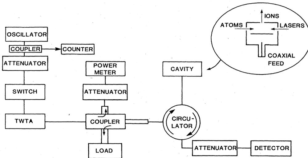
FIG. 1. Block diagram of the microwave system with the cross section of the cavity shown in the inset. Waveguide connections (=), coaxial connections (—).
