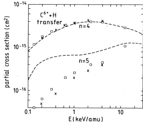
FIG. 5. Partial cross sections for transfer into  $C^{5+} n=4$  and  $n=5$  orbitals in  $C^{6+} + H$  collisions. Results of the 33-state MO investigation (Ref. 12) are shown in dashed lines, results of the 35-state AO study (Ref. 11) are indicated by open squares, and the present results are given in crosses.
