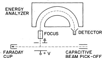
FIG. 1. Schematic of the experimental apparatus. The pulsed ion beam passes midway between the parallel plates. The target ions are accelerated at low energy toward a hemispherical analyzer and detector. Their time-of-flight is recorded.
