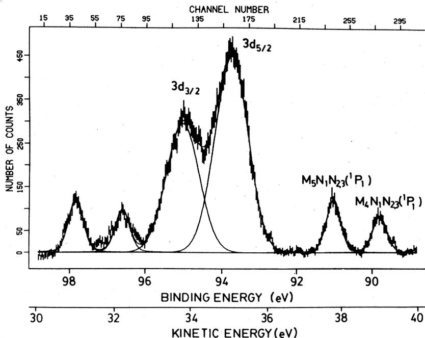
FIG. 1. The Kr  $3d$  and part of the  $MNN$  Auger spectrum taken at 130-eV photon energies, 75- $\mu\text{m}$  slits, and 50-eV pass energy.
