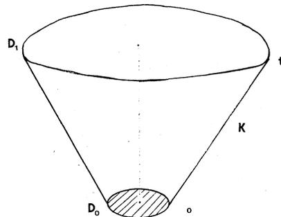
FIG. 1. Cone of influence for a circular disk of initial data of radius  $R$  called  $D_0$  at  $t=0$ . The phase velocity has constant magnitude  $c$ . At  $t$  the disk has spread to  $D_1$  which has the radius  $R+ct$ . Causality requires that  $u(\mathbf{x},t) \equiv 0$  for all  $(\mathbf{x},t)$  not in the cone of influence. The construction of spherical surfaces from each point is the Huygen's construction for data  $D_0$ .
