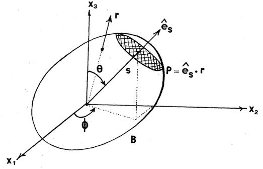
FIG. 3. Geometry of the three-dimensional Radon transform. The support of  $V$  is denoted as  $B$ ;  $\hat{e}_s = \hat{e}_s(\theta, \phi)$  is the unit vector in the scattered direction.
