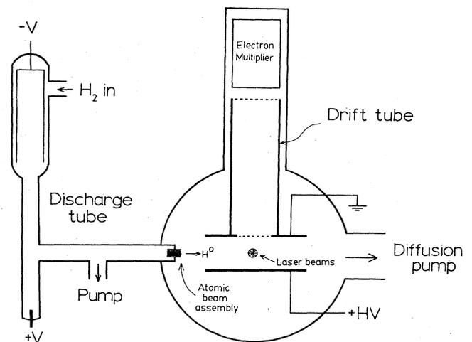
FIG. 1. Block diagram of the experimental setup.
