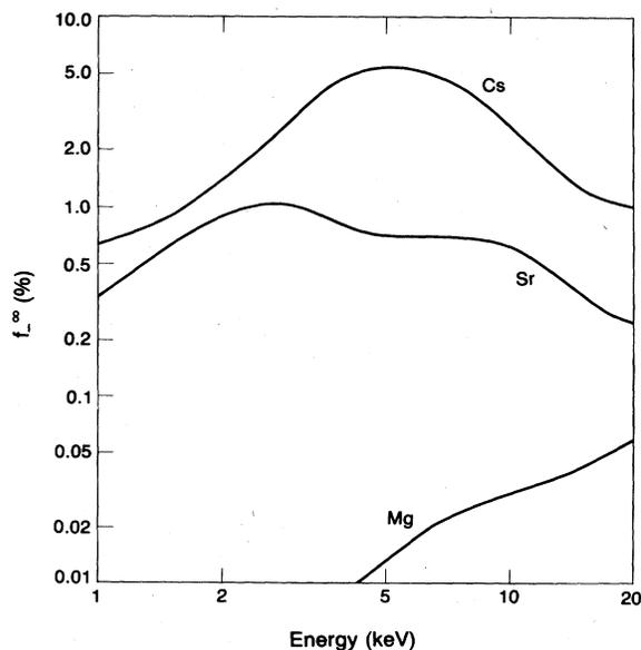
FIG. 6. Summary of  $f_{-}^{\infty}$  for Li ions in metal vapors.
