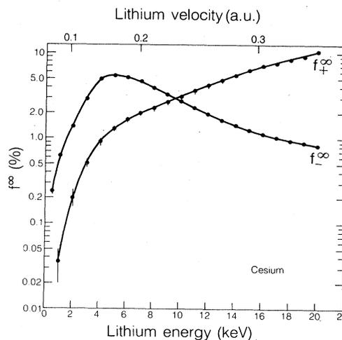
FIG. 5. Equilibrium charge-state fractions: Li in Cs vapor.
