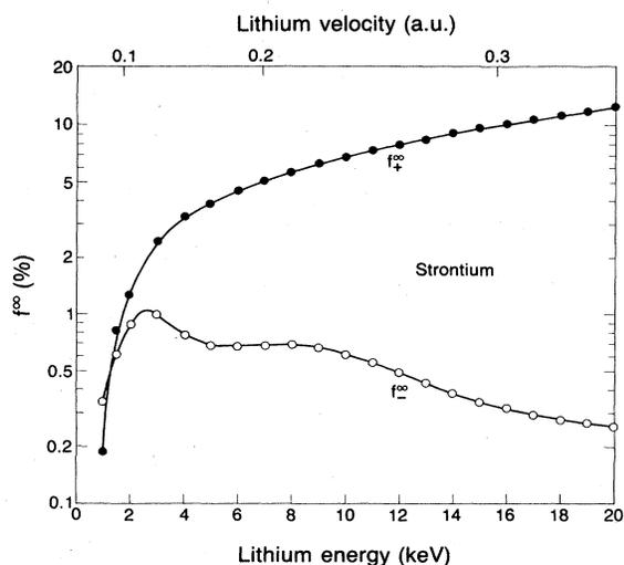
FIG. 4. Equilibrium charge-state fractions: Li in Sr vapor.
