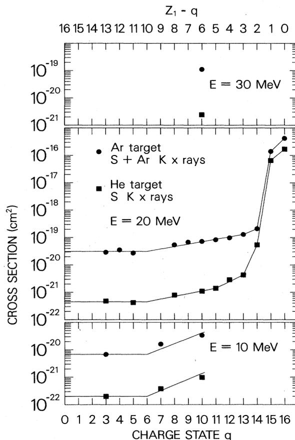
FIG. 2.  $K$ -x-ray production cross sections for  ${}_{16}\text{S}^{q+}$  on  ${}_{18}\text{Ar}$  and  ${}_{16}\text{S}^{q+}$  on  ${}_2\text{He}$  at  $E = 30, 20,$  and  $10$  MeV as a function of the projectile charge state  $q$  or the projectile electron number  $Z_1 - q$ . The curves are to guide the eye.
