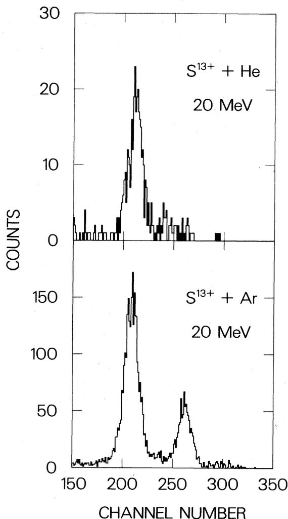
FIG. 1. Typical  $K$ -x-ray energy spectra for  ${}_{16}\text{S}^{13+} + {}_2\text{He}$  and  ${}_{16}\text{S}^{13+} + {}_{18}\text{Ar}$  collisions at 20 MeV.
