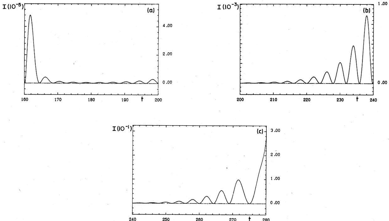
FIG. 5. Blowup of Fig. 4(a) indicating the fine structure of the interpulse domain: (a) decay of the pulse followed by (b) and (c) an exponential increase of the intensity with an oscillatory modulation.
