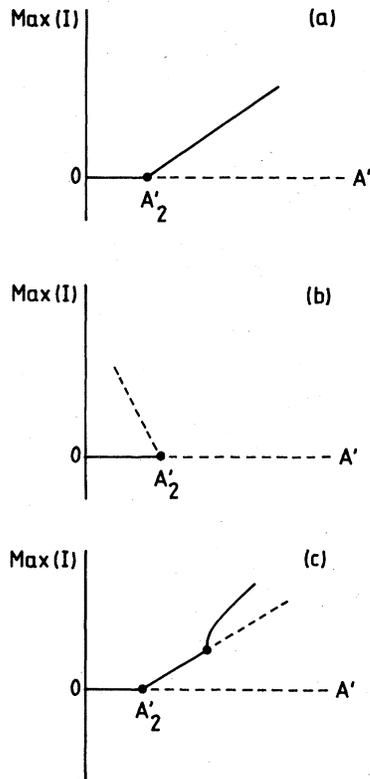
FIG. 6. Bifurcation diagram for the harmonic solutions. (a)  $al^2 - 1 < 0$  and  $d_{||}^2 - \bar{d}_{||}^2 al^2 > 0$ : supercritical bifurcation towards stable periodic solution. (b)  $al^2 - 1 > 0$  and  $d_{||}^2 - \bar{d}_{||}^2 al^2 \leq 0$ : subcritical bifurcation towards unstable periodic solution. (c)  $al^2 - 1 < 0$  and  $d_{||}^2 - \bar{d}_{||}^2 al^2 < 0$ : supercritical bifurcation followed by a secondary bifurcation towards quasiperiodic solutions.
