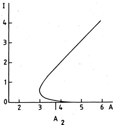
FIG. 1. Stationary intensity vs pump parameter of the amplifying atoms as given by (2) and (5).
