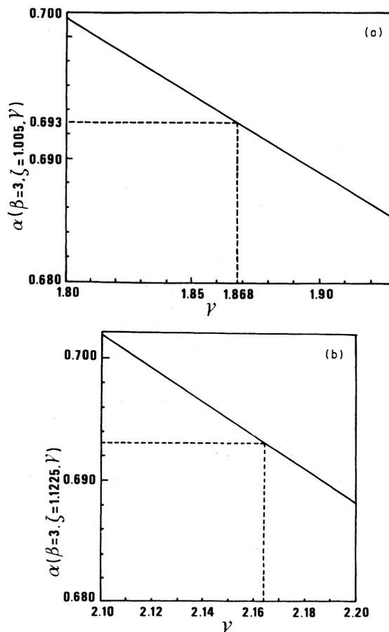
FIG. 7. (a) The variation of  $\alpha(\beta=3, \xi, \gamma)$  vs  $\gamma$  for our deduced two-particle potential function. From this figure we obtain  $\gamma=1.868$ , which corresponds to  $\alpha=0.6930$ . (b) The variation of  $\alpha(\beta=3, \xi, \gamma)$  vs  $\gamma$  for the Lennard-Jones potential function. From this figure  $\alpha=0.6930$  corresponds to  $\gamma=2.164$ .
