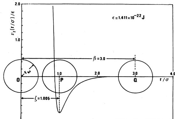
FIG. 5. Schematic representation of the interaction between two helium atoms, in which the two-particle potential function  $v_2$  has been normalized, i.e.,  $v_2 = -u_2$ , where  $v_2$  is expressed in units of J.
