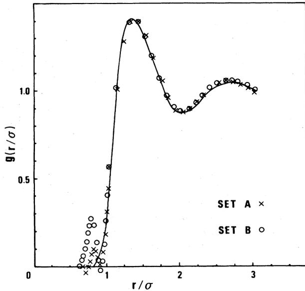
FIG. 1. Variation of the radial distribution function  $g_2(r/\sigma)$  as a function of  $r/\sigma$ . The solid line indicates the neutron scattering experimental result of Henshaw (Ref. 12). We fit this curve by the stated curve-fitting techniques and two sets of coefficients from Table I: set A,  $\times$ ; set B,  $\circ$ .
