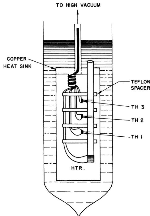
FIG. 2. Experimental schematic. Th1, Th2, Th3 are thermometers (1/8 W Allen-Bradley resistors). The heater at the bottom of tube is made of Karma wire (nominal resistance 700  $\Omega$ ). The top of the stainless-steel tube is open directly to the helium bath.
