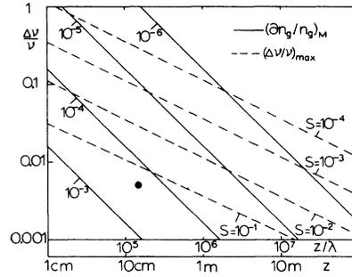
FIG. 2. Diagram to evaluate the accuracy [Eq. (31)] of a direct group-velocity measurement as a function of bandwidth  $\Delta \nu$  and sample length  $z$ . Valid are readings below that dotted line [Eq. (29)] which corresponds to the actual second-order derivative  $S = \lambda^2 |\partial^2 n_p / \partial \lambda^2|$ . A second scale for actual sample lengths has been provided which is valid for 1- $\mu$  wavelength. The dot refers to the example (Sec. V).
