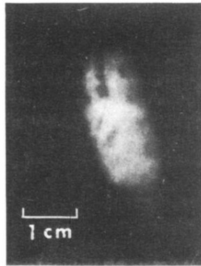
FIG. 1. Photograph of the helium crystal used in most of the measurements taken by Bragg reflection of neutrons.
