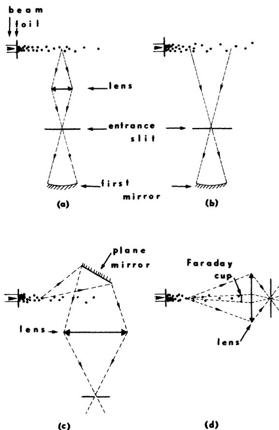
FIG. 1. Experimental settings (not to scale). (a) and (b): "side-on" systems; (c) and (d): "end-on" mirror and lens systems.
