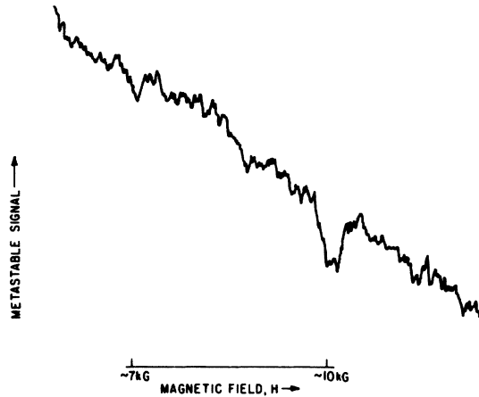
FIG. 4. Typical intermediate-field quenching curve for \text{Li}^7 .
