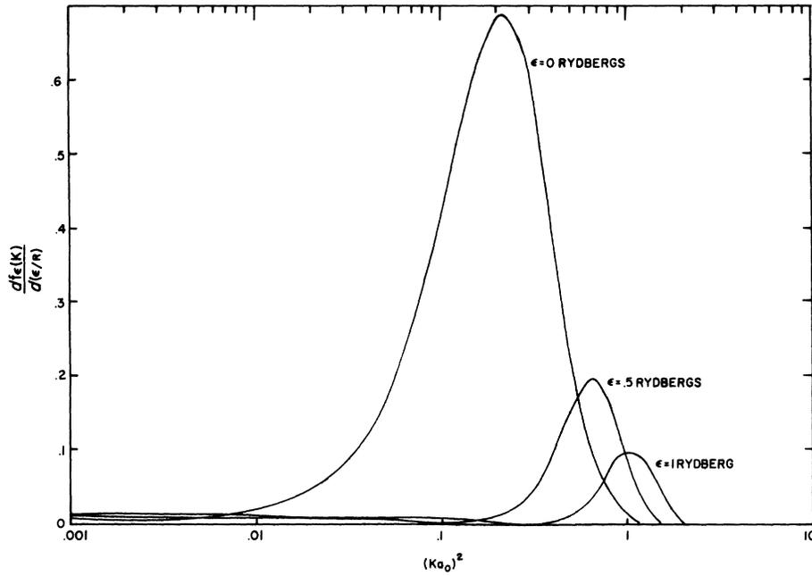
FIG. 2. Generalized oscillator strength of K for the  $4s \rightarrow \epsilon p$  transition.
