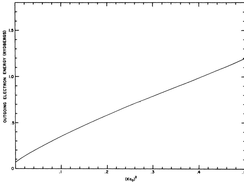
FIG. 3. Trajectory of the minimum in the generalized oscillator strength of Na for the  $3s \rightarrow \epsilon p$  transition.
