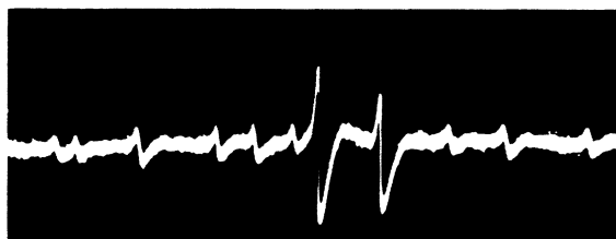
FIG. 1. Cathode-ray trace of the J=1-2 , K=0 and K=1 transitions of \text{AsD}_3 , showing hyperfine structure due to ^{75}\text{As} nuclear coupling.
