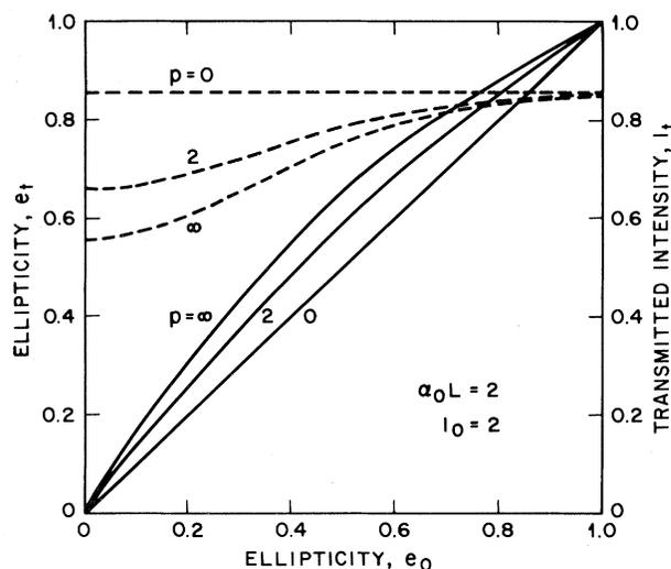
FIG. 2. Variation of the transmitted intensity  $I_t$  (dashed line) and the ellipticity  $e_t$  (full line) with the input ellipticity  $e_0$  for three values of the parameter  $p$  that is a measure of the collisional decay of Zeeman coherence.
