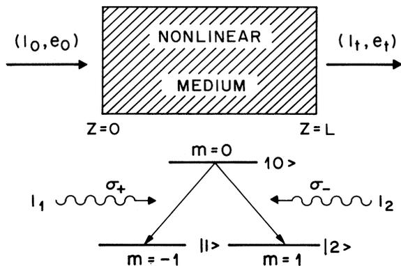
FIG. 1. Schematic illustration of the geometry, notation, and transition scheme for propagation of an elliptically polarized optical field in a three-level system, modeling  $J=1 \rightarrow J=0$  transition.
