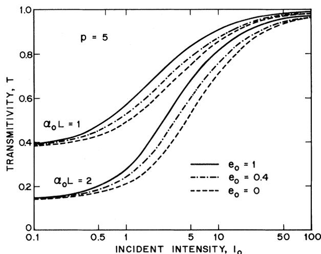
FIG. 3. Transmittivity  $T = I_t/I_0$  as a function of the incident intensity  $I_0$  (normalized to the saturation intensity) for three values of the ellipticity  $e_0$ . The cases  $e_0 = 0$  and  $e_0 = 1$  correspond to linear and right-circular polarizations, respectively.
