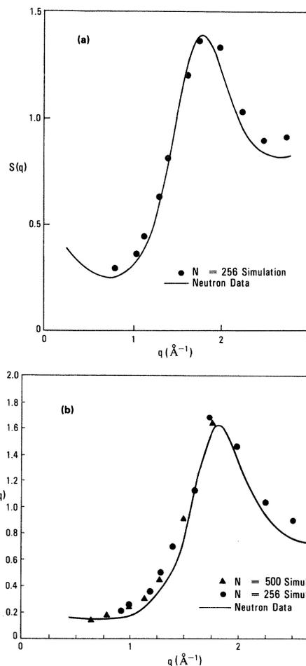
FIG. 1. Comparison of measured and calculated static structure factors  $S(q)$  at (a)  $n^* = 0.482$  and (b)  $n^* = 0.628$ .
