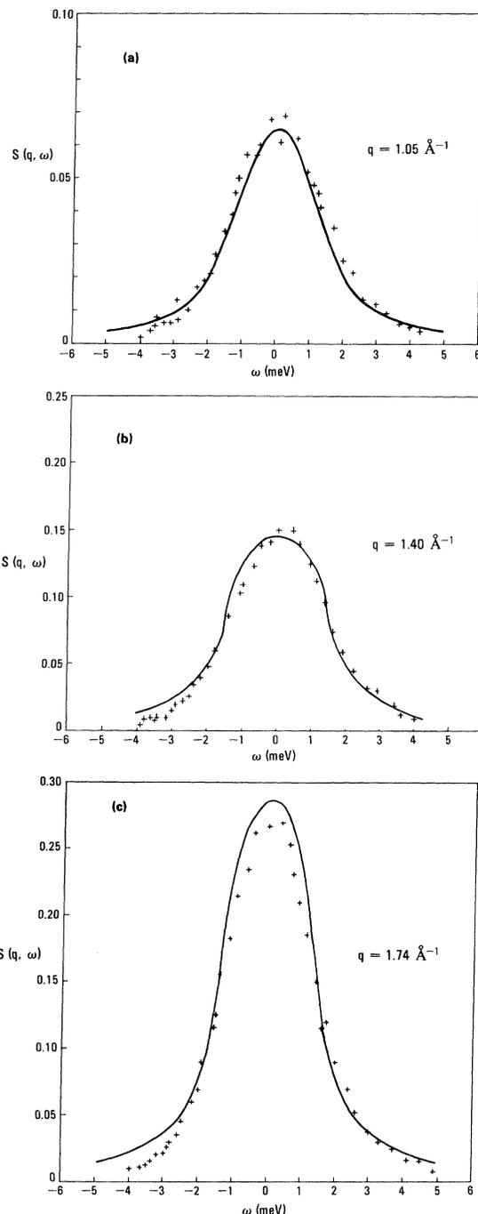
FIG. 4. (a) Comparison between calculated  $S(q, \omega)$  ( $N = 256$ ) and measured spectra at  $n^* = 0.482$ ,  $q = 1.05 \text{ \AA}^{-1}$ . (b) Comparison between calculated  $S(q, \omega)$  ( $N = 256$ ) and measured spectra at  $n^* = 0.482$ ,  $q = 1.40 \text{ \AA}^{-1}$ . (c) Comparison between calculated  $S(q, \omega)$  ( $N = 256$ ) and measured spectra at  $n^* = 0.482$ ,  $q = 1.74 \text{ \AA}^{-1}$ .
