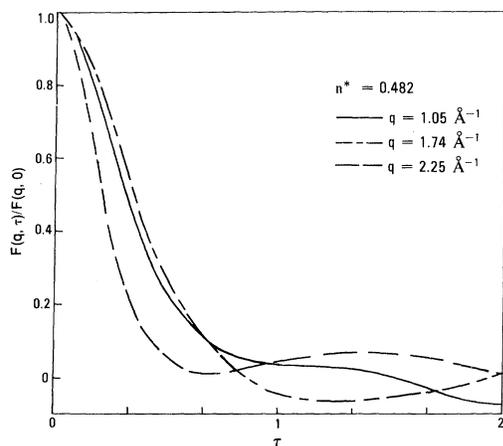
FIG. 2. Time dependence of the normalized intermediate scattering function  $F(q, \tau)/F(q, 0)$  at several wave numbers for  $n^* = 0.482$ . ( $q = 1.05, 1.74, 2.25 \text{ \AA}^{-1}$ .) Note use of  $\tau = \sigma(m/\epsilon)^{1/2}$  as the time variable.
