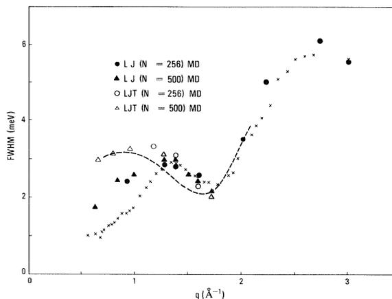
FIG. 6. Variation of  $\Delta\omega$  with  $q$  at  $n^*=0.628$ . Crosses are neutron data corrected for resolution; dashed line is from hard-sphere kinetic theory; closed and open circles are molecular-dynamics simulations for 256 particles using the  $V_{LJ}$  and  $V_{LJT}$  potentials, respectively; closed and open triangles are molecular-dynamics simulations for 500 particles using the  $V_{LJ}$  and  $V_{LJT}$  potentials, respectively.
