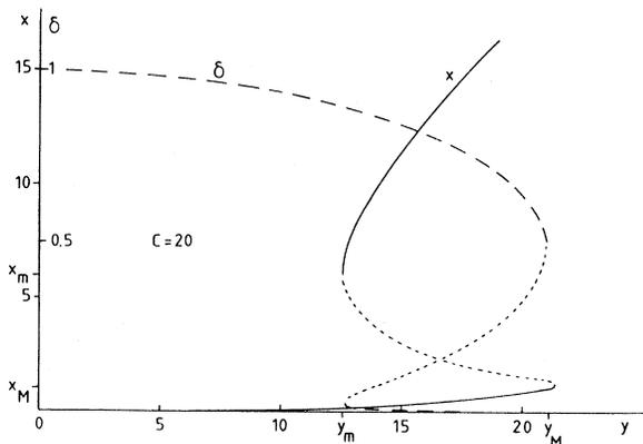
FIG. 1. Steady-state output-field amplitude ( $x$ ) and atomic population ( $\delta$ ) vs input-field amplitude.
