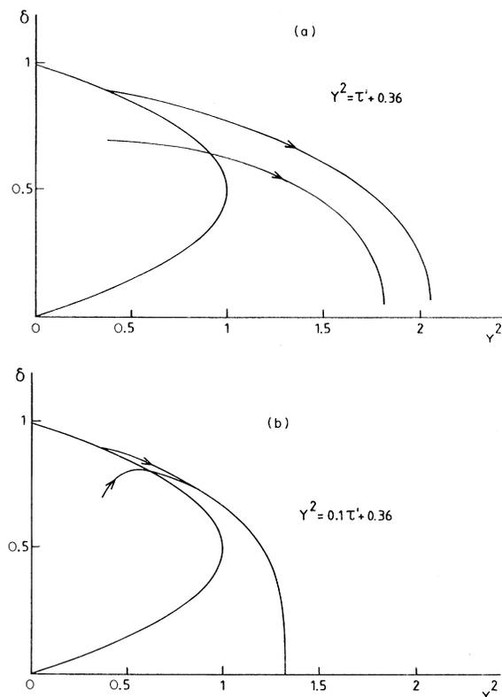
FIG. 3. Influence of the initial condition on the dynamic response of the system. (a) For  $Y^2 = \tau' + 0.36$  the two curves remain different. (b) For  $Y^2 = 0.1\tau' + 0.36$  the two curves differ only for very short times.
