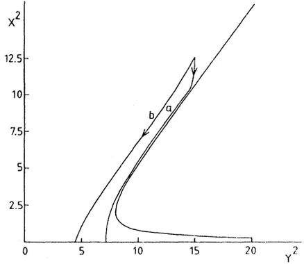
FIG. 5. Down switching under influence of an output intensity decreasing according to  $Y^2(\tau') = Y^2(0) - \alpha\tau'$ . Initial conditions:  $Y^2(0) = 15$  and  $X^2(0) = 12.5$ . Sweeping velocities:  $\alpha = 0.1$  for curve a and  $\alpha = 1.0$  for curve b.
