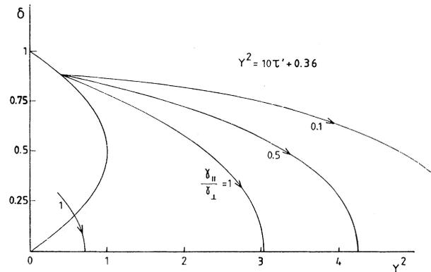
FIG. 7. Examples of subcritical ( $Y < 1$ ) and supercritical ( $Y > 1$ ) transitions; influence of the ratio  $\gamma_{||}/\gamma_{\perp}$  for a sweeping velocity ten times greater than in Fig. 8. Two initial conditions are  $Y^2(0) = 0.36$  with  $\delta(0) = 0.9$  and  $0.3$ .
