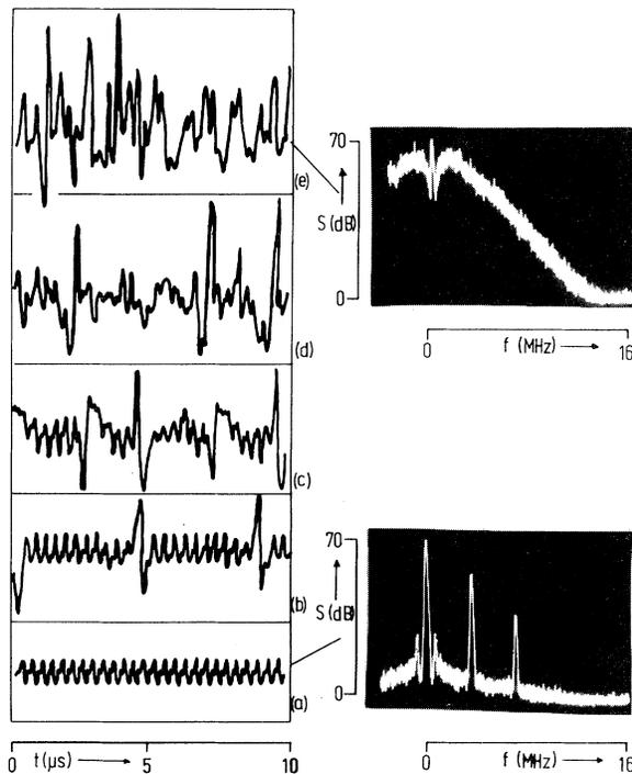
FIG. 4. Time dependence of laser output as the control parameter (mirror tilting angle) is varied from stable oscillatory state (a) to chaotic state (e). Spectra corresponding to (a) and (e) are also shown. (Observed  $-9$  MHz from the gain line center.)
