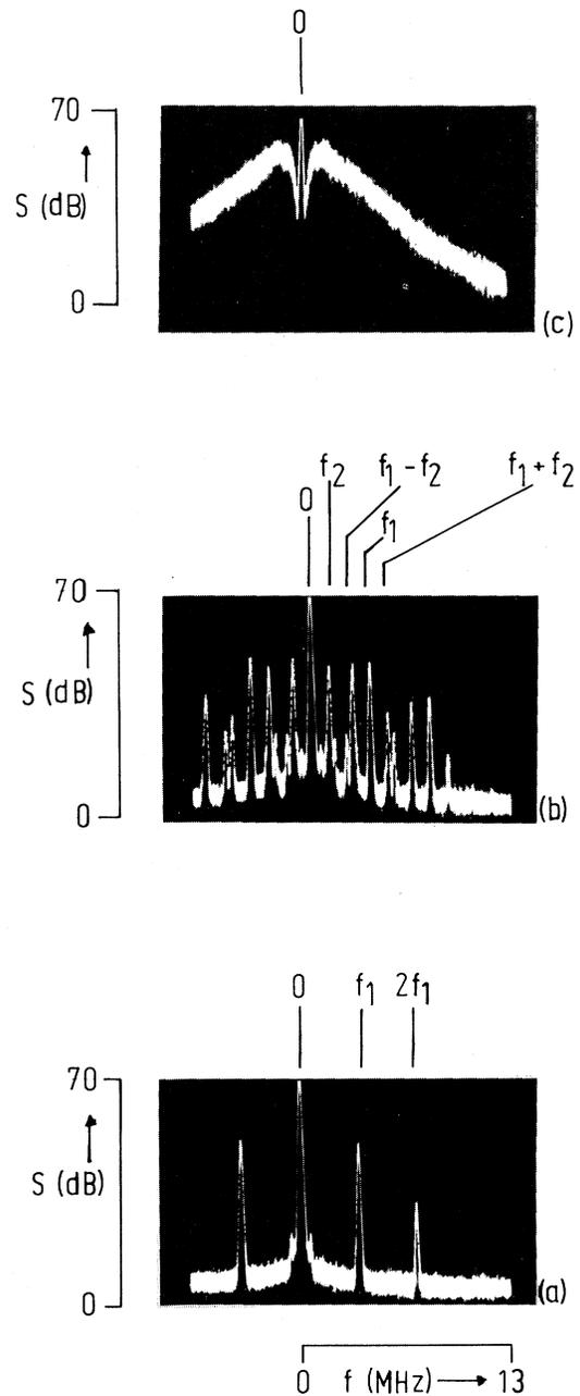
FIG. 3. Starting from single-mode oscillation, tilting of one resonator mirror leads to an oscillation  $f_1$  [(a)] followed by a two-periodic state  $f_1, f_2$  [(b)] followed by chaos [(c)]. Laser frequency offset -2 MHz.
