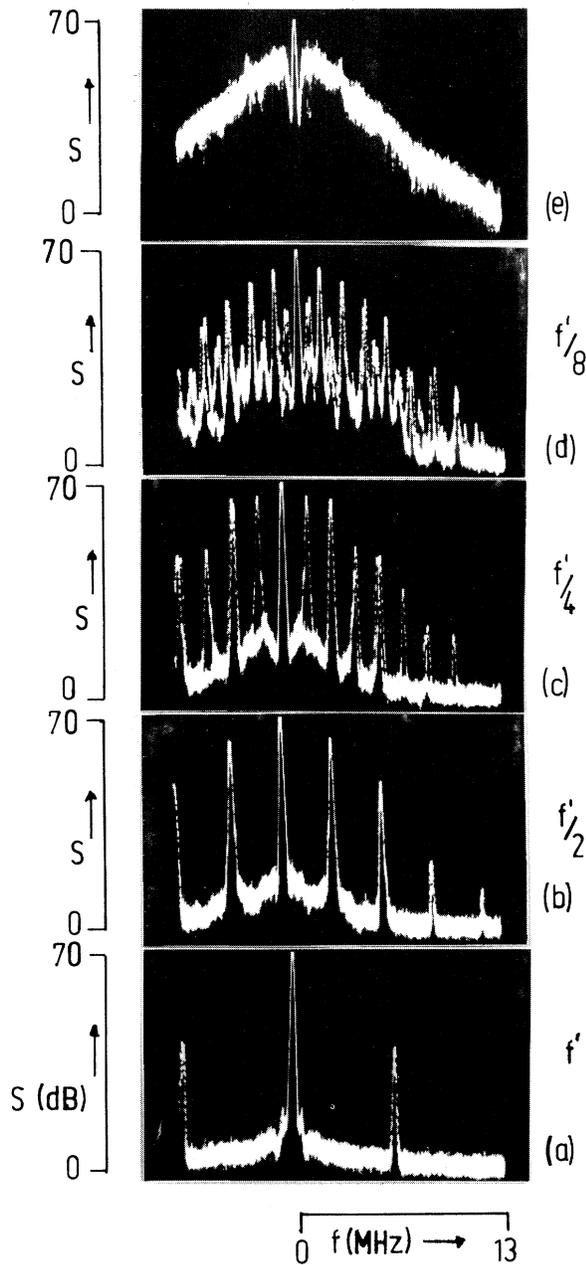
FIG. 2. Starting from single-mode oscillation, tilting of one resonator mirror leads to an oscillation  $f'$  [(a)], period doubling [ $f'/2$ , (b)], period doubling [ $f'/4$  (c)], period doubling [ $f'/8$ , (d)], and chaos [(e)]. Laser frequency offset from the gain line center +5 MHz. Spectrum is not given correctly in all measurements below 1 MHz due to lower cutoff frequency of detector amplifier. ( $S$ , relative intensity of oscillation;  $f$ , oscillation frequency.)
