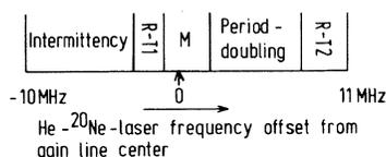
FIG. 6. Different routes to chaos appearing at different laser frequency settings when all other laser parameters are held constant. Intermittency, see Fig. 4. RT 1, Ruelle-Takens sequence, Fig. 3;  $M$ , transitional sequence described in text; period doubling, Feigenbaum sequence, Fig. 2; RT 2, Ruelle-Takens sequence, Fig. 5.
