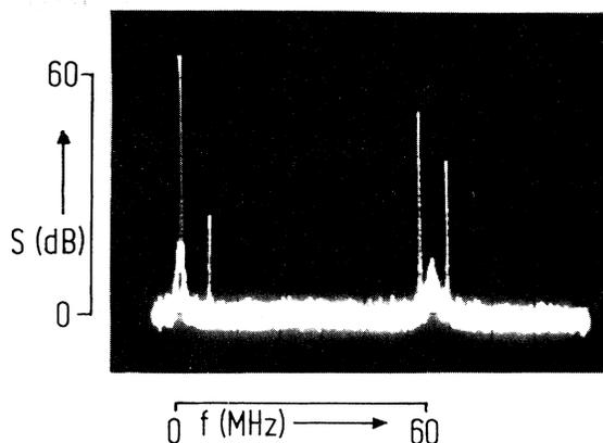
FIG. 7. RF spectrum of the laser output from 0 to 100 MHz showing two different mode beats at approximately the resonator free-spectral range of 60 MHz. The difference of the beat frequencies is probably due to the laser medium dispersion. Low-frequency oscillation is equal in frequency to the difference of the mode beats. [Mirror tilting corresponds to Fig. 2(a)]. Incoherent signals are probably due to modes below threshold.
