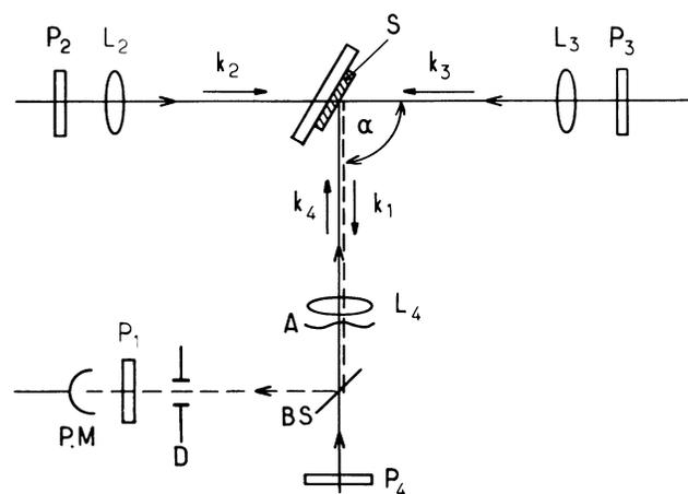
FIG. 1. Schematic diagram of DFWM setup for optical phase conjugation.  $S$  = sample,  $L$  = lens,  $P$  = polarizer,  $A$  = aberrator,  $D$  = variable aperture,  $BS$  = beamsplitter. For the data shown in this paper,  $\alpha = 3^\circ$  and the pump beams are normal to the sample surface.
