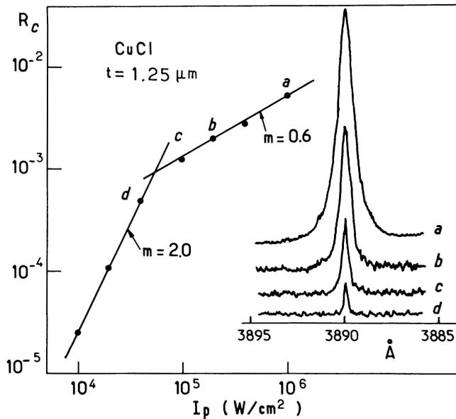
FIG. 3. Peak value of the phase-conjugate reflectivity  $(R_c)_{\max}$  as a function of pump beam intensity. The lines correspond to  $(R_c)_{\max} \propto I_p^m$ . The inset shows the spectral dependence of  $R_c$  near the TPA wavelength. The labeled spectra correspond to the identically labeled points in the plot of  $(R_c)_{\max}$ .
