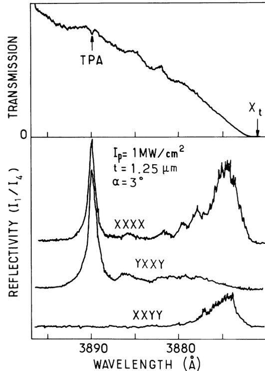
FIG. 2. Laser wavelength dependence of optical-phase-conjugation signal for a  $1.25\text{-}\mu\text{m}$ -thick sample at  $T=1.8 \text{ K}$  and  $I_p=1 \text{ MW/cm}^2$ . The four polarization components are in the order phase-conjugate wave (1), pump (2), pump (3), probe (4). The  $x$  direction is orthogonal to the scattering plane and  $y$  is in this plane. The upper trace shows the transmission of one pump beam.  $X_T$  corresponds to the wavelength of the transverse exciton.
