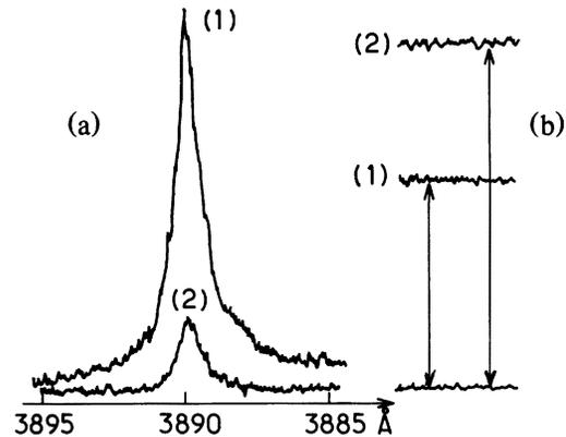
FIG. 4. (a) Spectra of the phase-conjugate reflected beam when an aberrator is inserted at A in Fig. 1; (b) magnitude of the signal observed when the probe beam is retroreflected by a plane mirror interchanged with the sample. In the traces labeled (1) or (2) the measured polarization is parallel or perpendicular, respectively, to that of the original probe beam before its passage through the aberrator.  $\alpha = 3^\circ$ .
