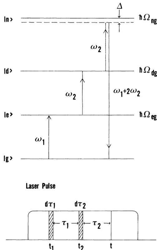
FIG. 1. Schematic diagram of the doubly resonant third-harmonic generation process. Calculation of the nonlinear dipole moment  $\vec{P}^{nl}(t)$  is performed by dividing the time period before  $t$  into many small time intervals.
