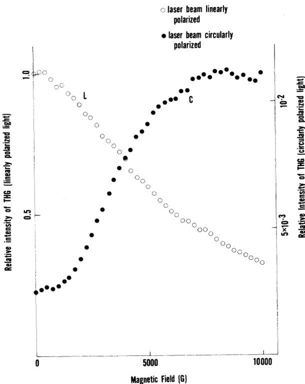
FIG. 4. Third-harmonic generation in I<sub>2</sub>. C, with a circularly polarized light. L, with a linearly polarized light. Note the difference between the scales of the two curves. At  $H \sim 7500$  G, third harmonic generated by a circularly polarized light is approximately 3% of that produced by a linearly polarized light under similar conditions.
