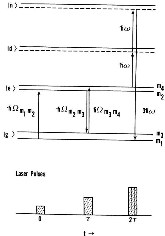
FIG. 3. Process of resonant third-harmonic generation in free atom or molecule associated with the photon-echo process. Zeeman splitting is exaggerated in this diagram.
