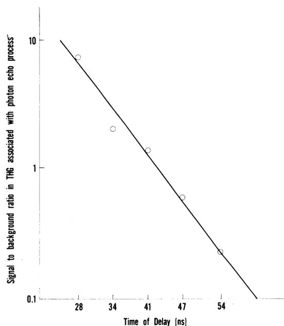
FIG. 8. Ratio of the intensity of THG associated with the photon-echo process plotted as a function of the time of delay between the first and the third pulse.
