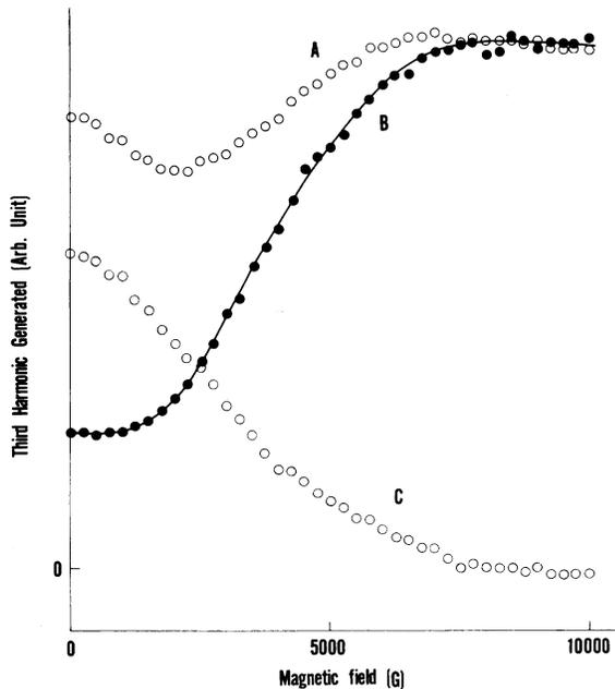
FIG. 6. *A*, intensity of the harmonic generation with all three pulses present. *B*, background signal produced by the pulses individually. *C*, difference between *A* and *B* is the intensity of THG associated with the photon-echo process. Wavelength is 5668 Å. The time delay between the pulses are  $\tau_{12} = \tau_{23} = 17$  ns.
