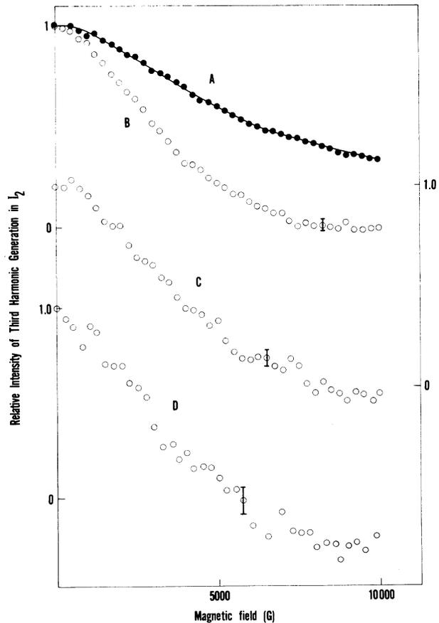
FIG. 7. Normalized intensity of THG. *A*, with a linearly polarized laser pulse. *B*, THG associated with photon-echo process with  $\tau_{12} = \tau_{23} = 17$  ns. *C*, same as *B* except that  $\tau_{12} = \tau_{23} = 20.4$  ns. The scale of the intensity is shown on the right-hand side of the diagram. *D*, same as *B* except that  $\tau_{12} = \tau_{23} = 23.6$  ns.
