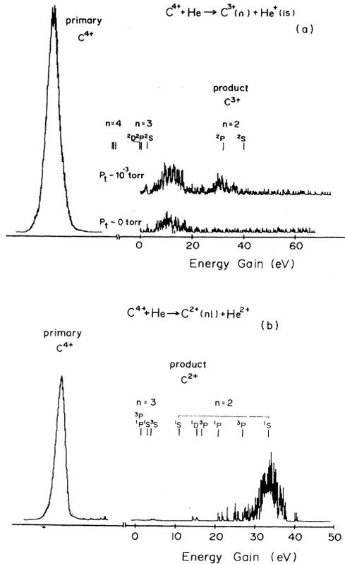
FIG. 6. (a) Typical energy spectrum of  $C^{3+}$  ions in the forward direction from the  $C^{4+} + He$  collision at 0.31 keV/amu. (b) Typical energy spectrum of  $C^{2+}$  ions in the forward direction from the  $C^{4+} + He$  collision at 0.31 keV/amu.
