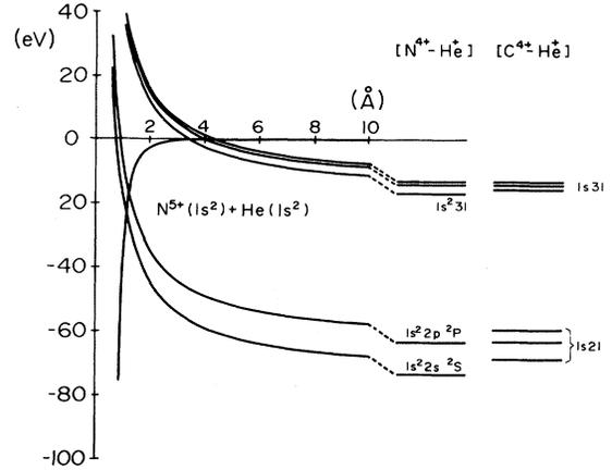
FIG. 5. Diabatic potential curves for the one-electron-capture process,  $N^{5+}(1s^2) + He \rightarrow N^{4+}(1s^2 nl) + He^+(1s)$ , and energy diagrams for channels of one-electron capture into  $N^{4+}(1s^2 nl)$  and  $C^{4+}(1s nl)$  levels.
