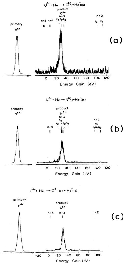
FIG. 2. (a) Typical energy spectrum of  $\text{O}^{5+}$  ions in the forward direction from the  $\text{O}^{6+} + \text{He}$  collision at 0.33 keV/amu. (b) Typical energy spectrum of  $\text{N}^{5+}$  ions in the forward direction from the  $\text{N}^{6+} + \text{He}$  collision at 0.30 keV/amu. (c) Typical energy spectrum of  $\text{C}^{5+}$  ions in the forward direction from the  $\text{C}^{6+} + \text{He}$  collision at 0.46 keV/amu.
