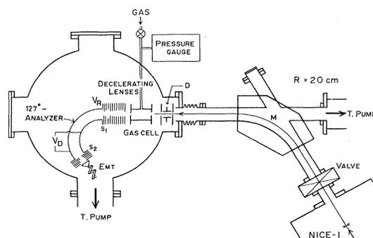
FIG. 1. Schematic view of the apparatus used for translation-energy spectroscopy.
