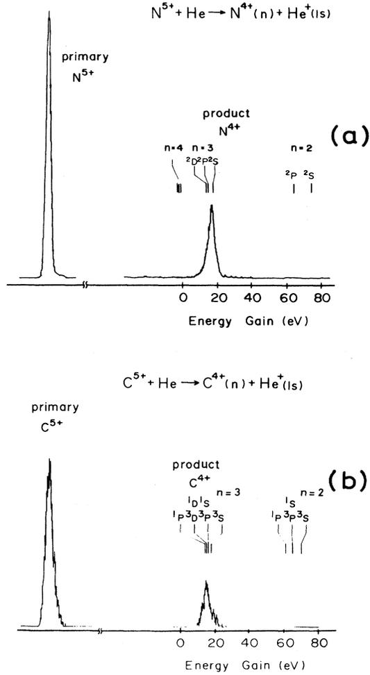
FIG. 4. (a) Typical energy spectrum of  $N^{4+}$  ions in the forward direction from the  $N^{5+} + He$  collision at 0.33 keV/amu. (b) Typical energy spectrum of  $C^{4+}$  ions in the forward direction from the  $C^{5+} + He$  collision at 0.38 keV/amu.
