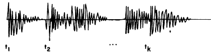
FIG. 4. Schematic representation of E(t) for nonstationary chaotic emissions occurring at the Poisson times \{t_k\} .
