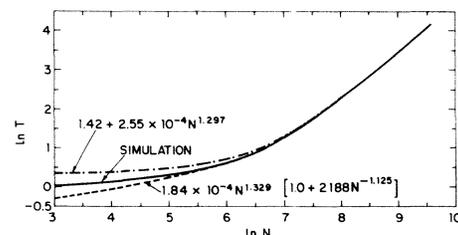
FIG. 7. Results of fitting the dependence of the rms thickness ( $T$ ) on the number of particles ( $N$ ) by scaling relationship of the form  $T = AN^\epsilon + B$  and  $T = AN^{\epsilon'}(1 + BN^{-\alpha})$ . Simulation results are the average results for nine deposits on 1000 original  $1d$  surface sites.
