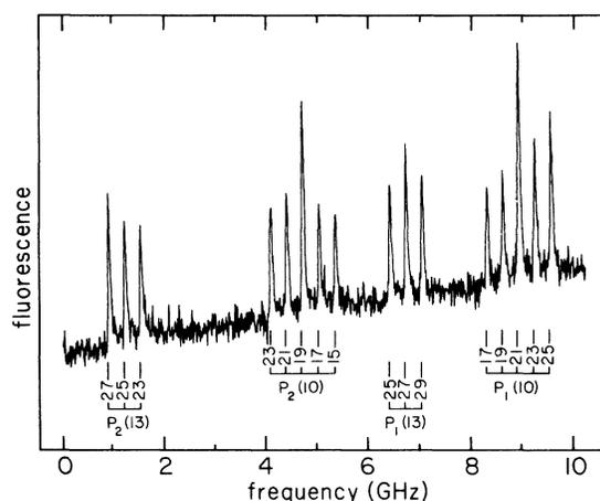
FIG. 1. Fluorescence vs Doppler-shifted laser frequency (with arbitrary origin) for a part of the (0,1) band of the  $B^2\Sigma_u^+ - X^2\Sigma_g^+$  system of  $N_2^+$ . Hyperfine components are labeled by  $2F''$ . Total data accumulation time was 17 min.
