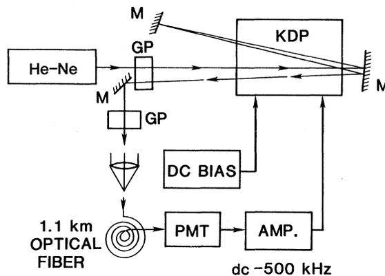
FIG. 1. Experimental layout: He-Ne laser; Glans prisms (GP); KDP, crystal; mirrors (M); photomultiplier (PMT).
