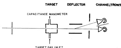
FIG. 1. Schematic layout of target and detectors.
