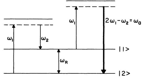
FIG. 1. Schematic of level configuration and the interaction of the pump fields at frequencies  $\omega_1$  and  $\omega_2$  in the generation of the CARS signal at frequency  $\omega_a$ .
