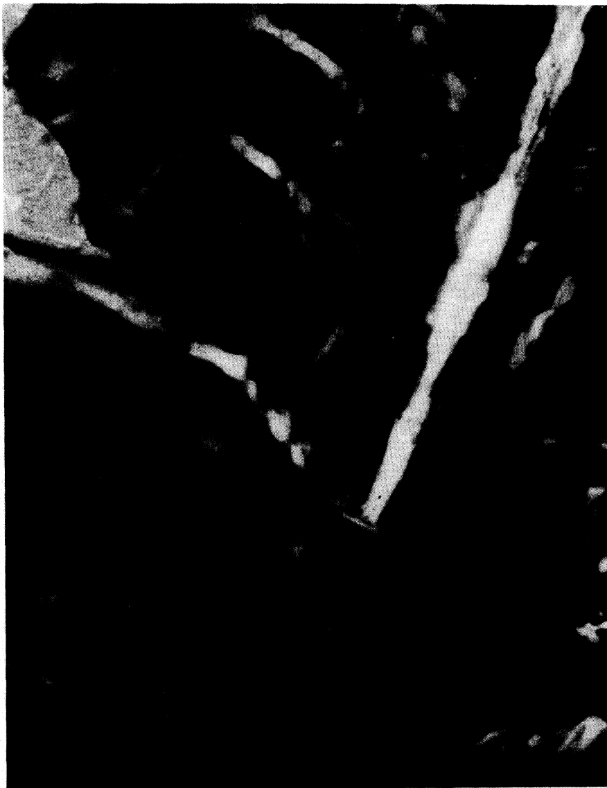
FIG. 2. BPI-II transition in sample no. 2. The light areas are BP II growing into the BPI.
