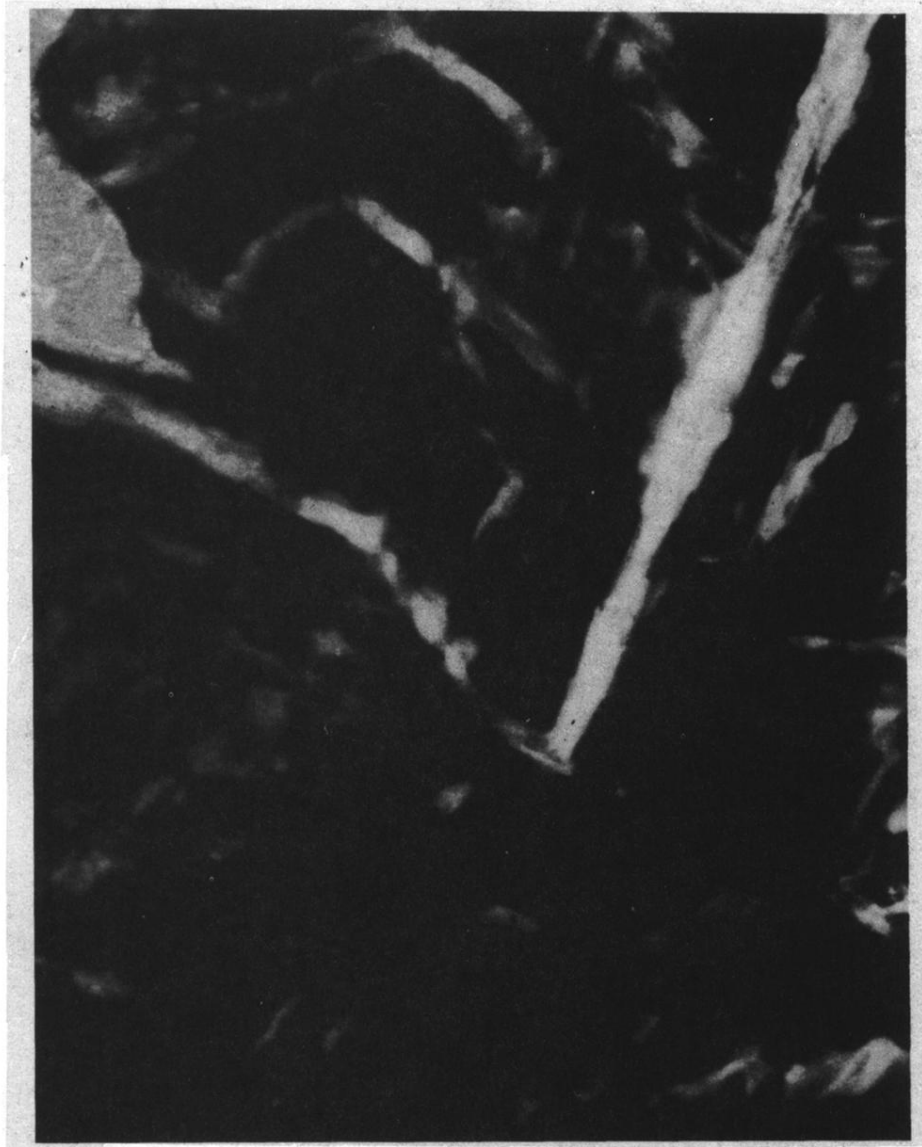
FIG. 2. BPI-II transition in sample no. 2. The light areas are BPII growing into the BPI.
