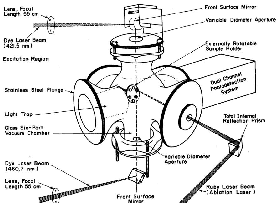
FIG. 1. Schematic view of laser ablation chamber.
