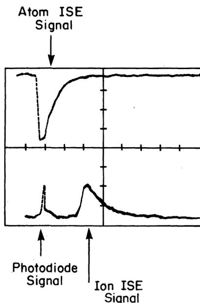
FIG. 2. Laser-intensified spontaneous-emission signals arising from an ablation plasma (1.2  $\mu$ sec after ablation). The upper trace corresponds to the ISE signal from strontium atoms (at 460.7 nm) while the lower trace corresponds to the ISE signal from strontium ions (at 421.6 nm). The first pulse on the lower trace arises from a photodiode that monitors one of the dye lasers. Time scales are 20 nsec/division.
