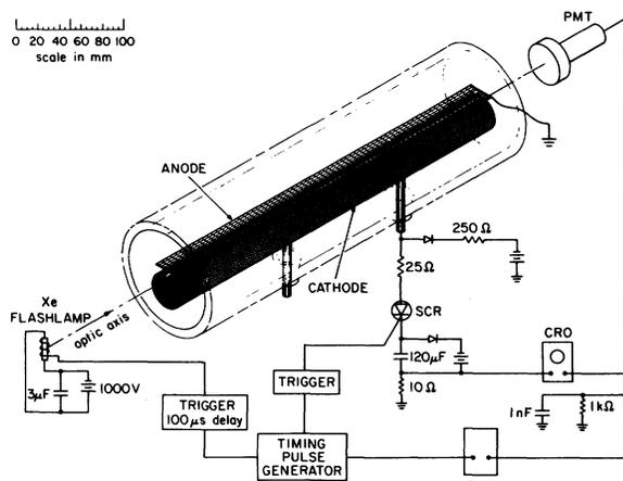
FIG. 1. Isometric drawing, approximately to scale, of the hollow cathode tube with a schematic of the accompanying electronics.
