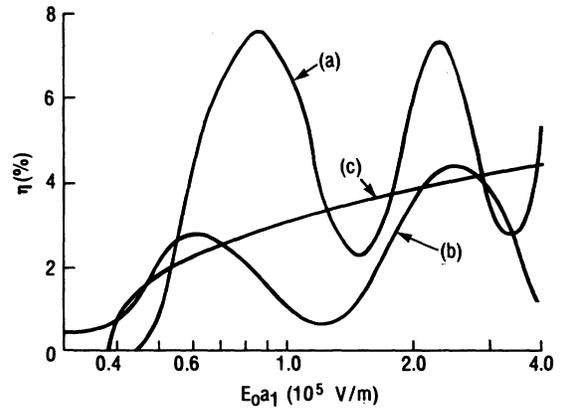
FIG. 1. Average electron efficiency vs electric field amplitude  $a_1 E_0$  for (a) "exact" Gaussian model, (b) pendulum model, and (c) phase-space model. The electron velocity is  $v_0 = 3.08 \times 10^7$  m/s.
