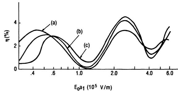
FIG. 3. Efficiency vs electric field amplitude for a variety of electron velocities in the pendulum model: (a)  $v_0 = 3.06 \times 10^7$  m/s, (b)  $v_0 = 3.07 \times 10^7$  m/s, and (c)  $v_0 = 3.08 \times 10^7$  m/s.
