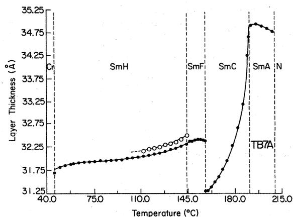
FIG. 8. Layer spacing of the smectic phases of TB7A as a function of temperature, shown by filled circles. The open circles are calculated from the strongest peak corresponding to a different value of  $d$ .
