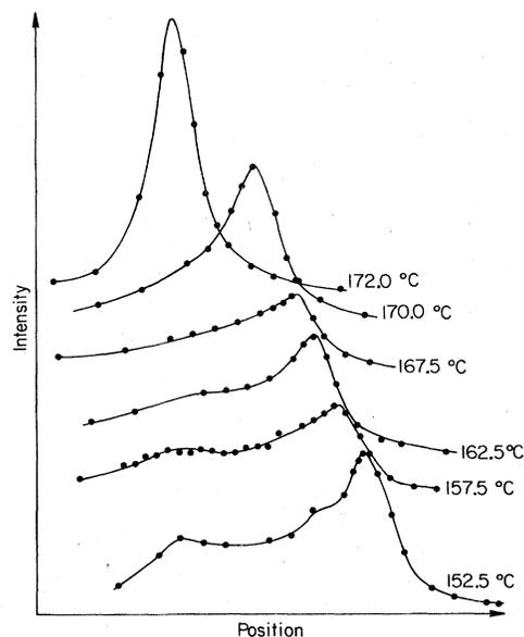
FIG. 17. The growth of asymmetry and development of secondary peaks in the Bragg reflections from the Sm-C phase of TB5A as the temperature is lowered.
