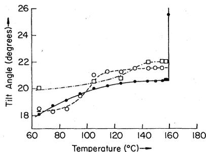
FIG. 15. Variation of the tilt angle with temperature in the Sm-H phase of TB8A. The filled circles are calculated from the measured  $d$ ; the open circles and squares, from the difference in the readings of the rocking scale. The lines are drawn as a guide to the eye.
