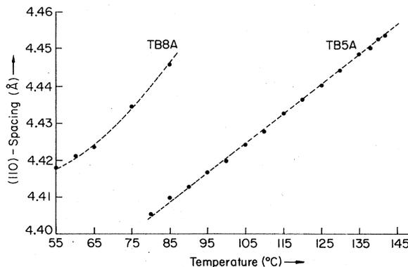
FIG. 14. (110) spacing of the Sm-H phase of TB5A and TB8A as a function of temperature. The lines are drawn as a guide to the eye.
