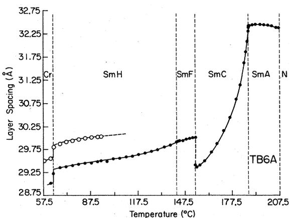
FIG. 7. Layer spacing of the smectic phase of TB6A as a function of temperature, shown by filled circles. The open circles correspond to the strongest peak from the domains with different layer thickness.
