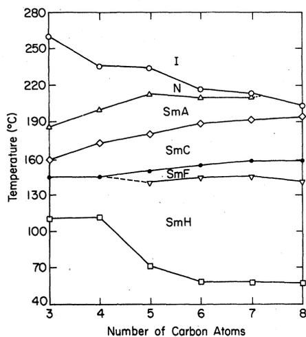
FIG. 2. Variation of the transition temperatures with the number of carbon atoms in alkyl chain.
