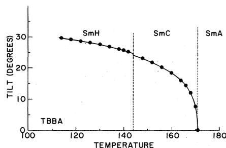
FIG. 11. The variation of the tilt angle in the smectic-C and - $H$  phases of TBBA, calculated from the measured value of  $d$ .
