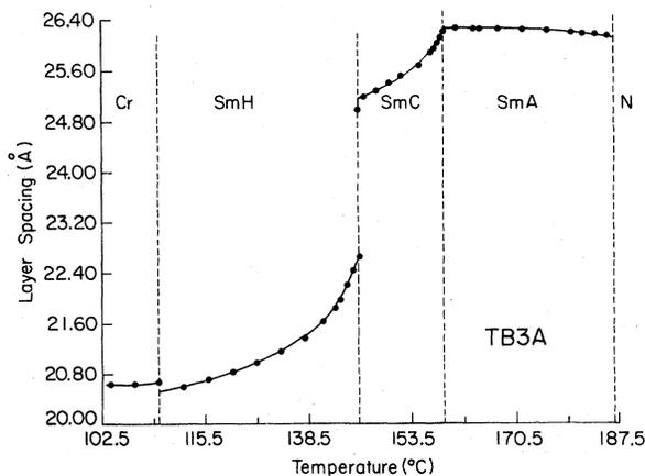
FIG. 4. Layer spacing of the smectic phases of TB3A as a function of temperature. The line joining the points is a guide to the eye.
