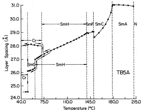
FIG. 6. Layer spacing of the smectic phases of TB5A as a function of temperature. The arrows show the direction of the temperature change. While cooling the monotropic smectic-G phase is observed.
