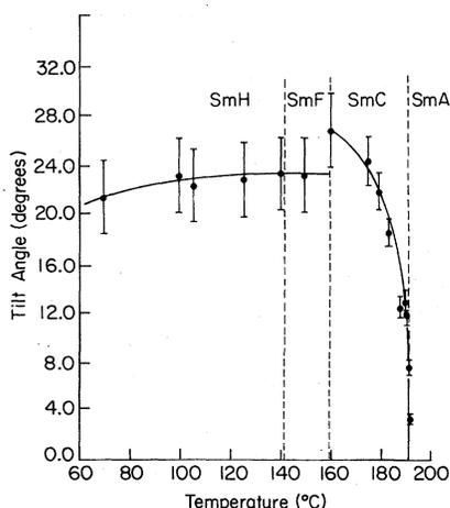
FIG. 16. Tilt angle as a function of temperature in the Sm-C, -F, and -H phases of TB8A measured by cono-scopy in the reflection mode.
