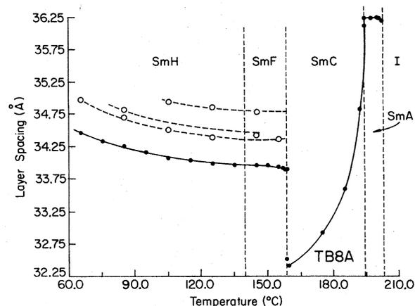
FIG. 9. Layer spacing of the smectic phase of TB8A as a function of temperature shown by filled circles. The open circles show the different values of  $d$  observed for different domains.
