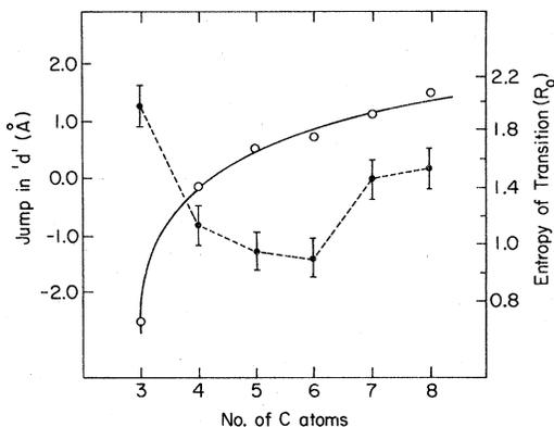
FIG. 13. The jump in the value of  $d$  (open circles) and the entropy change at the Sm-C to Sm-F/H transition (filled circles with error bars) versus the number of  $C$  atoms in the alkyl chain.
