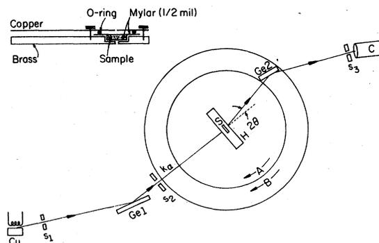
FIG. 1. Experimental set up for x-ray diffraction. S is the sample holder, S1, S2, and S3 are the slits, Ge1 and Ge2 are the Germanium crystals used as monochromator and analyzer, Cu is the source of x rays, C is the NaTlI scintillation counter. The sample holder is shown as the inset.
