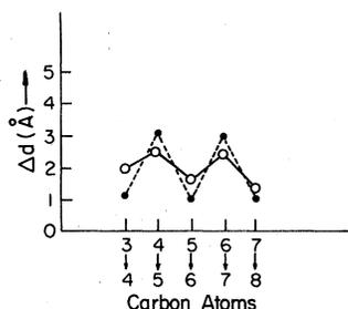
FIG. 10. The change in layer thickness of the Sm-A phase as the number of C atoms in alkyl chain is changed. This illustrates the even-odd effect. Open circles correspond to the measured change in  $d$  and filled circles to calculated change in the length of the molecule in transconfiguration.
