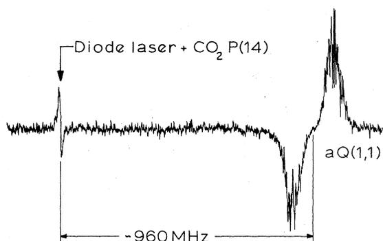
FIG. 4. Recorder tracing of observed  $\text{NH}_3$  spectra near  $11\text{-}\mu\text{m}$  wavelength. Two-ir-photon absorption  $(\nu_2, J, K) = (2^-, 1, 1) \leftarrow (0^-, 1, 1)$ , and a single-photon transition,  $(\nu_2, J, K) = (1^+, 1, 1) \leftarrow (0^-, 1, 1)$  referred to in the literature as  $aQ(1,1)$  (Ref. 12) are observed simultaneously. The phase of the two-photon transition is inverted with respect to the single-photon transition.
