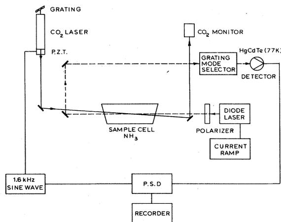
FIG. 1. Schematic of experimental apparatus.  $\text{CO}_2$  laser (ca. 15-W power) and diode laser (ca. 1 mW) beams propagating in nearly opposite directions are focused in a 10-cm-long cell containing  $\text{NH}_3$  gas. The transmitted intensity of the diode laser beam is measured with a cooled detector and a phase-sensitive detector. The  $\text{CO}_2$  laser is frequency modulated. The polarizer reduces  $\text{CO}_2$  power leakage into the diode laser system.
