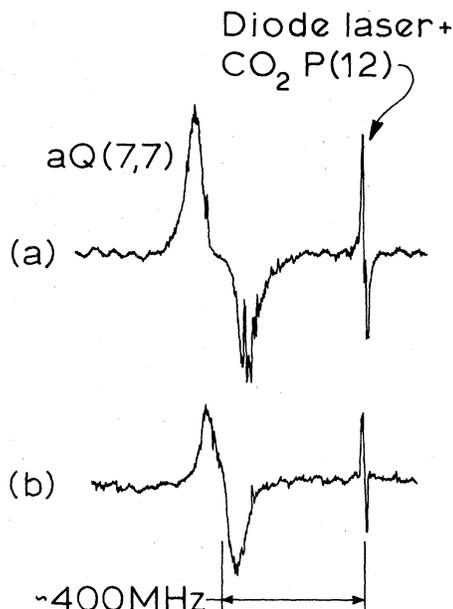
FIG. 5. Recorder tracings of the two-photon transition  $(\nu_2, J, K) = (2^-, 7, 7) \leftarrow (0^-, 7, 7)$  and the single-photon transition  $aQ(7,7)$  or  $(\nu_2, J, K) = (1^+, 7, 7) \leftarrow (0^-, 7, 7)$ . The single-photon and the two-photon transition have the same phase. Traces (a) and (b) are for  $\text{NH}_3$  pressures of about 0.1 and 0.4 torr, respectively.
