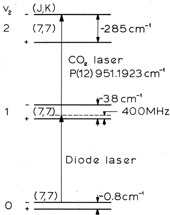
FIG. 3. Energy levels for the  $J,K = 7,7$  manifold, and observed two-photon transition.
