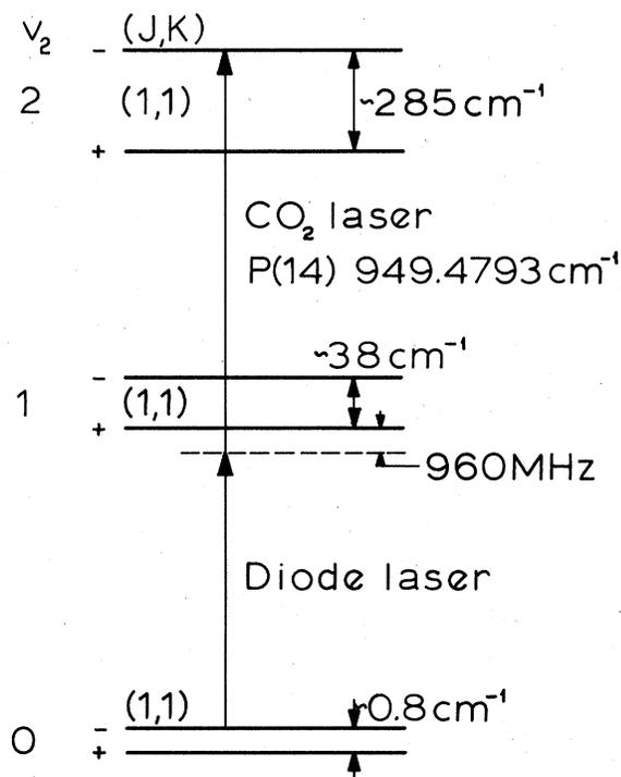
FIG. 2. Energy-level diagram (not to scale) showing the two-photon transition in the  $\nu_2$  band of NH<sub>3</sub> for the  $J,K = 1,1$  manifold. The intermediate level lies below the  $\nu_2 = 1$  inversion doublet.
