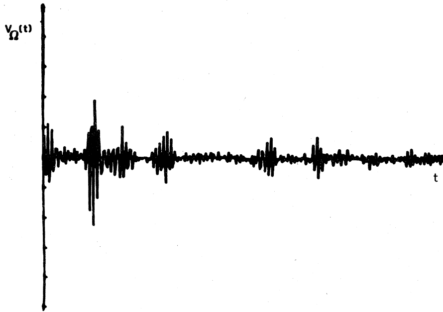
FIG. 1. Intermittent velocity signal obtained by Gagne. The plot shows high-pass filtered output of a hot-wire probe measuring the velocity in grid-generated turbulent flow.
