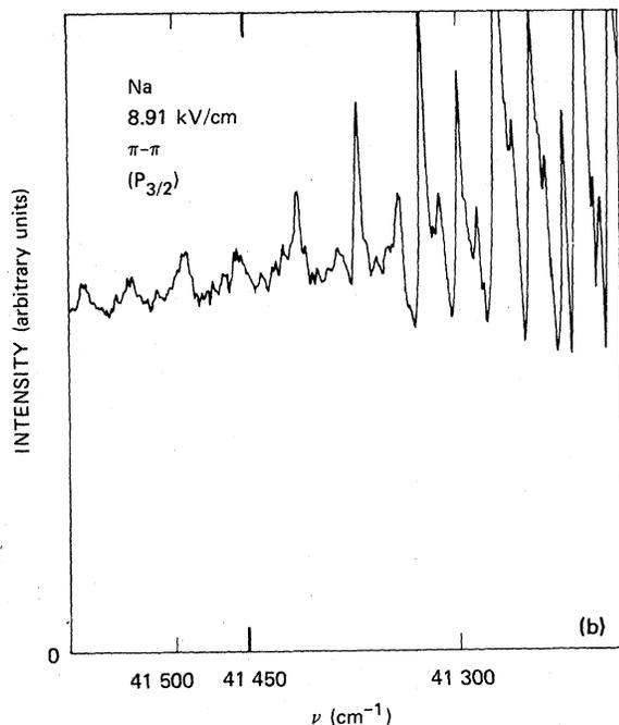
FIG. 3. (a), (b) Experimental photoabsorption signal in Na at an electric field strength of 8.91 kV/cm, obtained by resonant two-photon transition ( $\pi$ - $\pi$  polarization) via the  $3^2P_{1/2}$  intermediate state, and the  $3^2P_{3/2}$  intermediate state, respectively. The energy of  $41\,450\text{ cm}^{-1}$  corresponds to the zero-field ionization limit.
