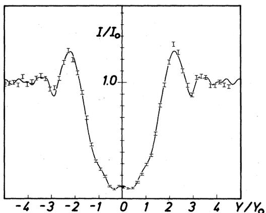
FIG. 4. Measured diffraction pattern of a 100  $\mu\text{m}$  Boron wire compared with the curve obtained from standard linear theory.
