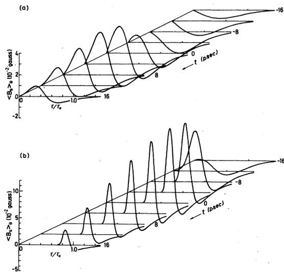
FIG. 5. Temporal changes in the radial distribution of magnetic field generated under the same conditions as in Fig. 3. (a)  $I_0 = 8 \times 10^{11}$  W/cm<sup>2</sup>; (b)  $I_0 = 3 \times 10^{12}$  W/cm<sup>2</sup>.
