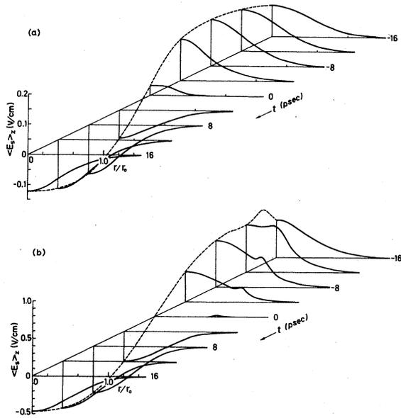
FIG. 4. Temporal changes in the radial distribution of axial electric field generated under the same conditions as in Fig. 3. (a)  $I_0 = 8 \times 10^{11}$  W/cm<sup>2</sup>; (b)  $I_0 = 3 \times 10^{12}$  W/cm<sup>2</sup>.
