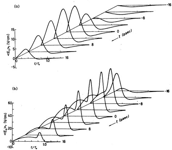
FIG. 3. Temporal changes in the radial distribution of radial electric field generated in atomic Na vapor. The incident Nd:YAG laser pulse is assumed to have the duration  $\tau = 28$  psec and the spot size  $r_0 = 152 \mu\text{m}$ . (a)  $I_0 = 8 \times 10^{11} \text{ W/cm}^2$ ; (b)  $I_0 = 3 \times 10^{12} \text{ W/cm}^2$ .
