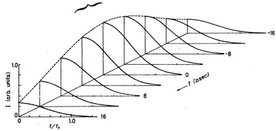
FIG. 7. Temporal change in the radial intensity distribution of the Gaussian laser beam used in the calculations. The peak intensity is normalized to unity at  $r=t=0$ .
