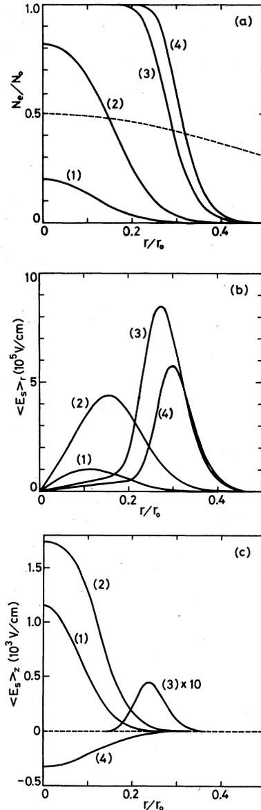
FIG. 6. Radial dependences of (a) multiphoton ionization rate, (b) radial electric field, and (c) axial electric field in He gas at the time  $t = (1) -5.5$ , (2)  $-3.8$ , (3)  $0$ , and (4)  $9.5$  psec. The incident Nd:YAG laser pulse is assumed to have the duration  $\tau = 28$  psec, the spot size  $r_0 = 15 \mu\text{m}$ , and the intensity  $I_0 = 1.5 \times 10^{15}$  W/cm<sup>2</sup>. The dashed line indicated in (a) represents the intensity distribution of the incident laser beam.
