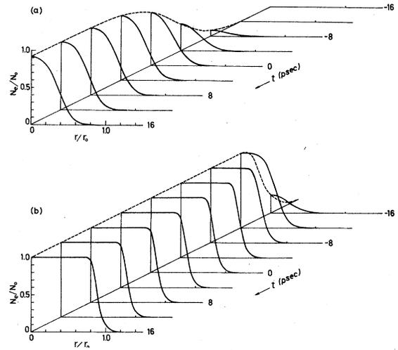
FIG. 2. Temporal changes in the radial dependence of multiphoton ionization rate in atomic Na vapor. The incident Nd:YAG laser pulse is assumed to have the duration  $\tau = 28$  psec. (a) Laser intensity  $I_0 = 8 \times 10^{11} \text{ W/cm}^2$ ; (b)  $I_0 = 3 \times 10^{12} \text{ W/cm}^2$ .
