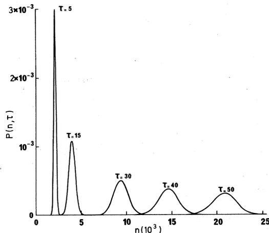
FIG. 1. Photon-number distribution for the nonlinear case ( $\chi=10^{-4}$ ) with the values of  $\tau=5, 15, 30, 40,$  and  $50$ . The distributions are normalized so that  $\sum_n P(n, \tau) = 1$ .
