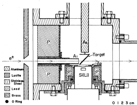
FIG. 1. Experimental arrangement in the target chamber: S, slit; P, lead shields;  $A_1$ , 10-mm-diam by 93-mm-long aluminum collimator;  $A_2$ , aluminum target holder;  $A_3$ , aluminum cap-ring with a 220- $\mu\text{m}$ -thick beryllium window.
