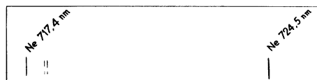
FIG. 5. Photograph of the laser light spectrum when it is tuned on the Fr D_2 resonance line. It is to be emphasized that in order to increase the precision of the wavelength measurement this picture has been taken using a dye laser oscillating on one single mode. This procedure has permitted us to distinguish between the two components due to the hyperfine splitting of the ground state.
