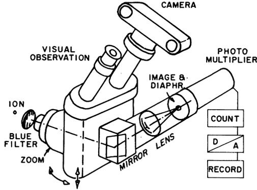
FIG. 1. Observation optics employing binocular microscope. The optics allowed simultaneous visual, photographic, and photoelectric observation of the stored ions. For a single ion the photon counting rate was  $\sim 10^4/s$ .
